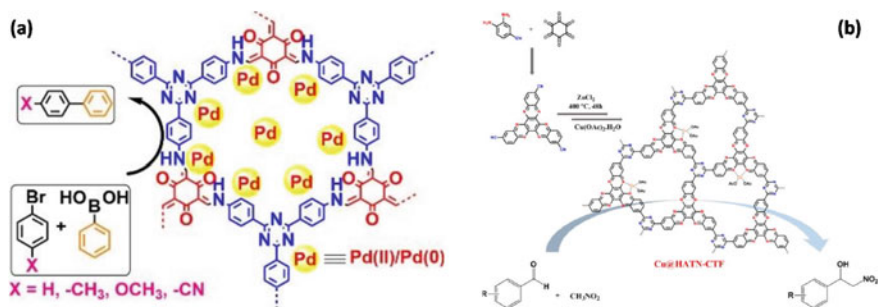
Fig. 11.9 a Synthetic procedure of Pd immobilized imine \beta -ketoenamine-linked COF and its use in coupling reactions [41] and b schematic representation of the synthesis of Cu@HATN-CTF and its catalytic application [42]
