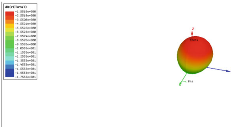
Fig. 4 3D polar plot of MANET antenna gain
