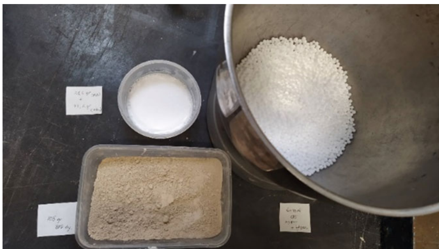
Fig. 5 Preparation before mixing/coating process with PVA/water binder
