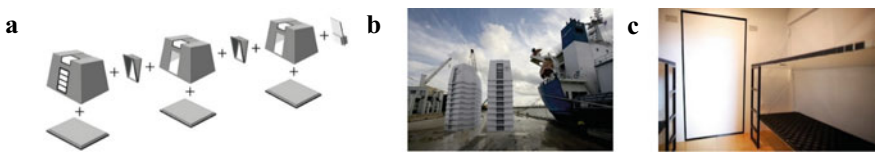
Fig. 1 a Separating component between building envelope and floor, b stacked building envelope like a cups of coffee, c bunk bed inside the shelter [14]
