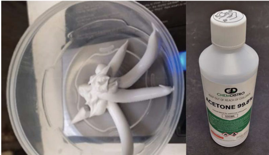
Fig. 3 PVA and acetone as a binder
