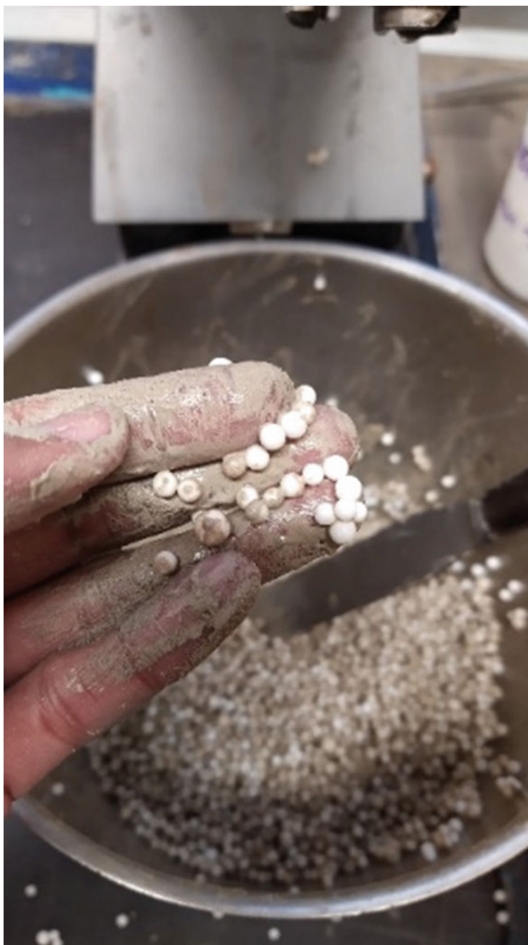
Fig. 4 Mixing/coating process with acetone–water binder
