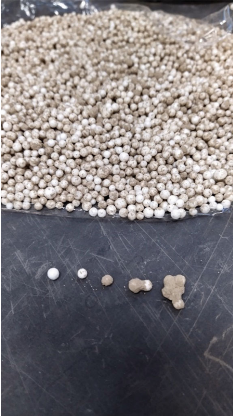
Fig. 6 Coated EPS beads with acetone–water binder
