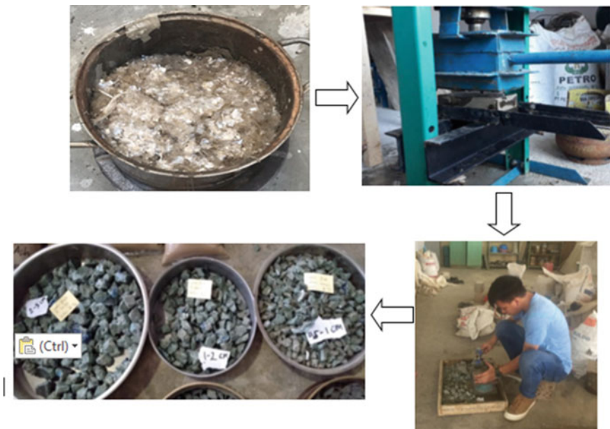
Fig. 1 Procedure on obtaining plastic waste aggregate
