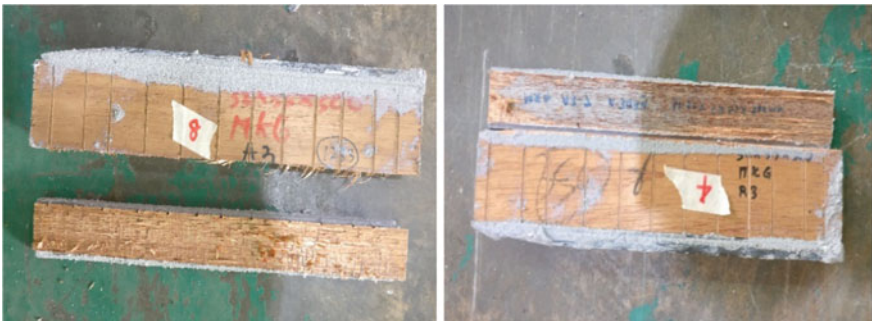
Fig. 8 Failure near to steel plate
