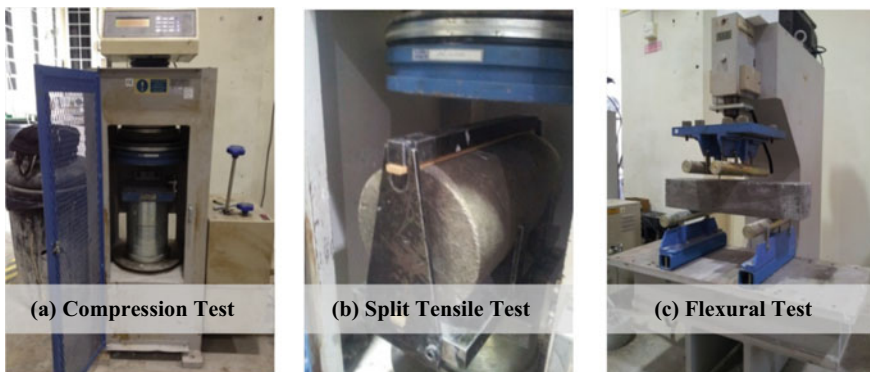
Fig. 3 Experimental setup for, a compression test, b splitting tensile test, c flexural test
