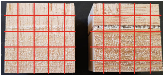
Fig. 11 Wood failure percentage was estimated as 10% at the 2nd layer of the sample
