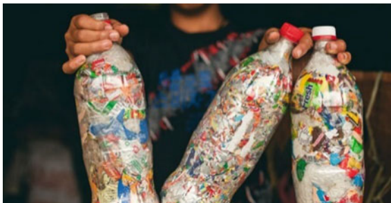
Fig. 7 Plastic filled plastic bottle bricks [34]
