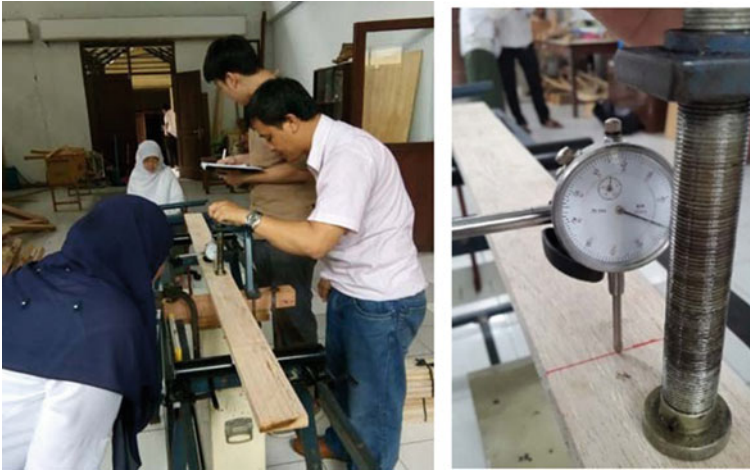
Fig. 5 (Left) Load test in progress using Panter and (Right) deflectometer for load and displacement reading
