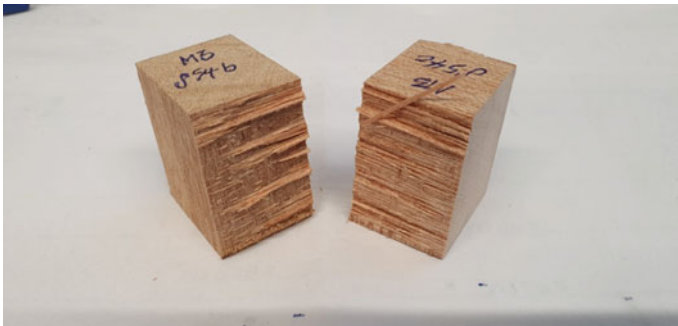
Fig. 8 Sample after block shear test
