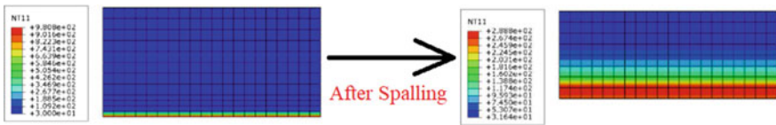
Fig. 7 Concrete before spalling (left) and after spalling (right)
