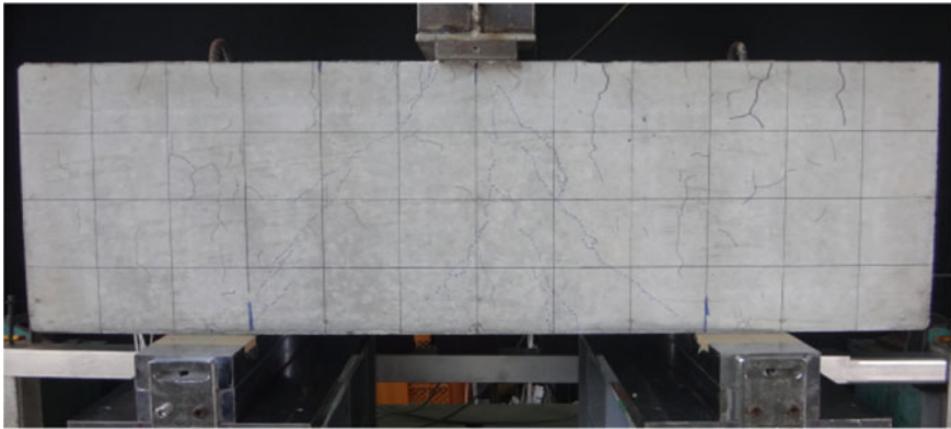
Fig. 2 Picture of the specimen after cracking
