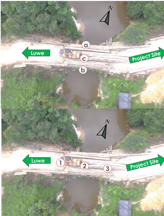
Fig. 8 Experimental static load test and dynamic load test
