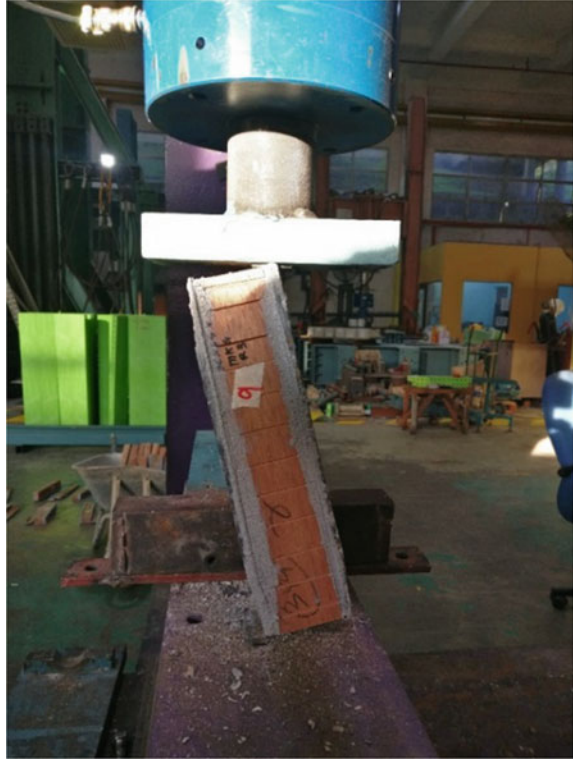
Fig. 4 Test set-up for the determination of shear strength according to BS EN 408 [10]
