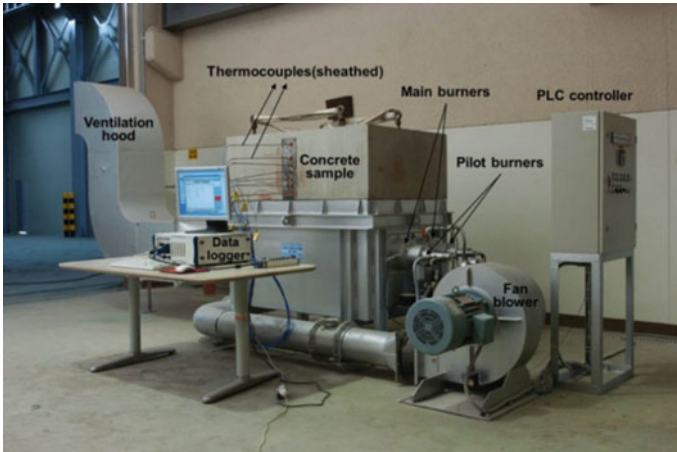
Fig. 1 Furnace used by Choi et al. [15] to imitate the RABT fire scenario
