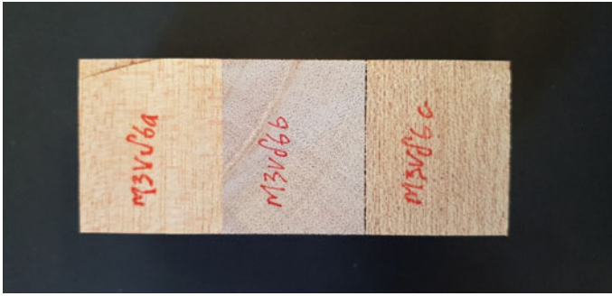
Fig. 9 Dry sample for a 3 layered of LRM CLT
