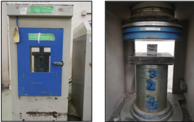
Fig. 2 Experimental set-up for compressive test
