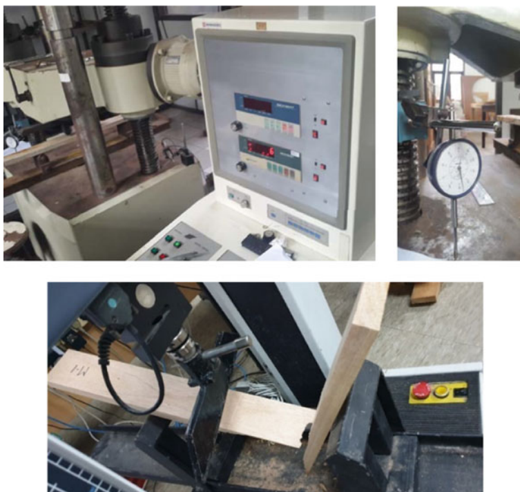
Fig. 6 (Top) Bending test execution using analogue UTM; (Bottom) test using digital UTM
