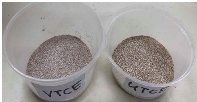
Fig. 1 The UTCE (right) and VTCE (left) after sieving through a No.30 mesh
