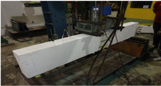
Fig. 1 Four point bending test setup—schematic (above) and actual (below)
