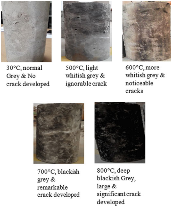
Fig. 7 Various aspects and crack formation of concrete (35% RGP) at prescribed temperatures
