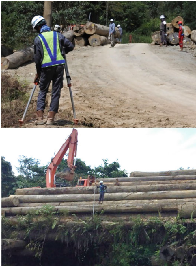
Fig. 9 Displacement measurement using auto-level
