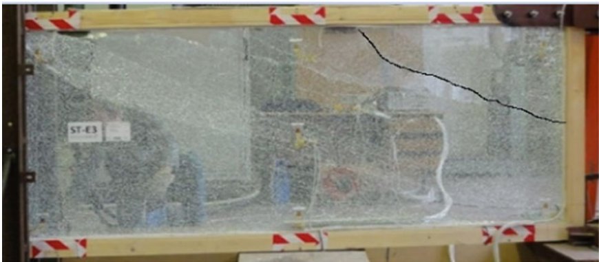
Fig. 10 Crack pattern for glass pane, a numerical test crack pattern, b experimental test crack pattern [3]
