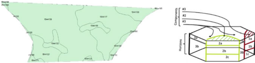
Fig. 2 (On the left side) Soil polygons in the area of analysis with their mukeys and (on the right side) structure of each soil polygon in SSURGO database (modified from [7])
