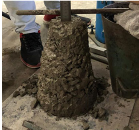
Fig. 1 Slump test for CF modified concrete
