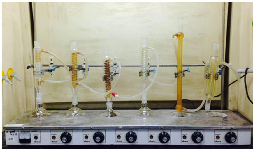
Fig. 1 Simple reflux apparatus with a control heating mantle
