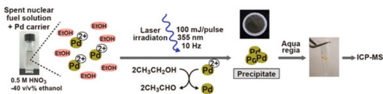
Fig. 3.9 Procedure of LIPF-based PM separation for the ICP-MS analysis of ^{107}\text{Pd} . Reprinted with permission from Ref. [7] (Copyright 2016 American Chemical Society)
