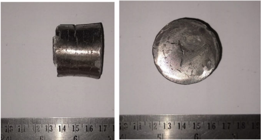
Fig. 5 Decanned induction sintered consolidate produced using 40 mm diameter die
