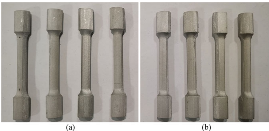
Fig. 4 Printed tensile specimens for mechanical investigations with two different metals: a Inconel 625, b 17-4 PH SS
