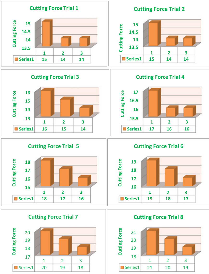
Fig. 12 Cutting force under dry wet and cryogenic condition in 9 trials
