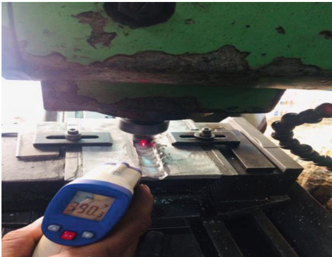
Fig. 3 Recording of temperature during FSP
