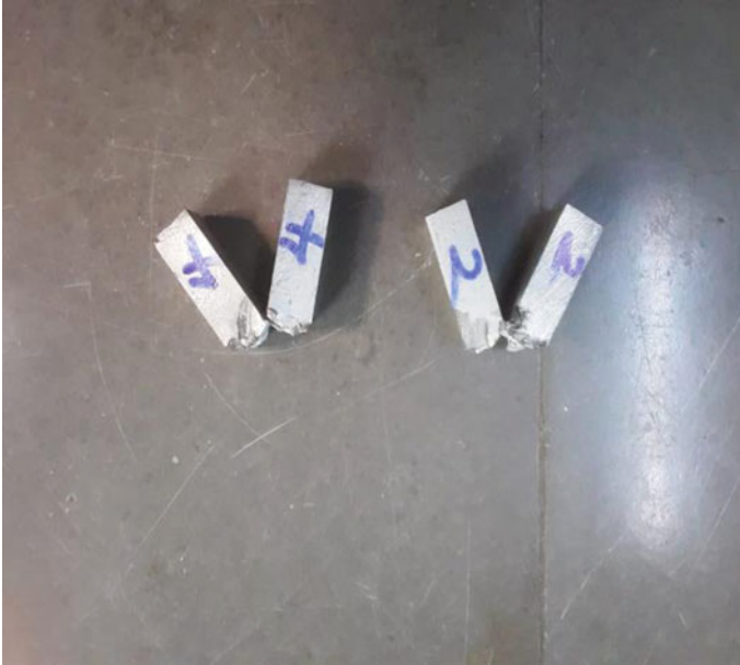
Fig. 8 Impact test samples of two pass and four pass
