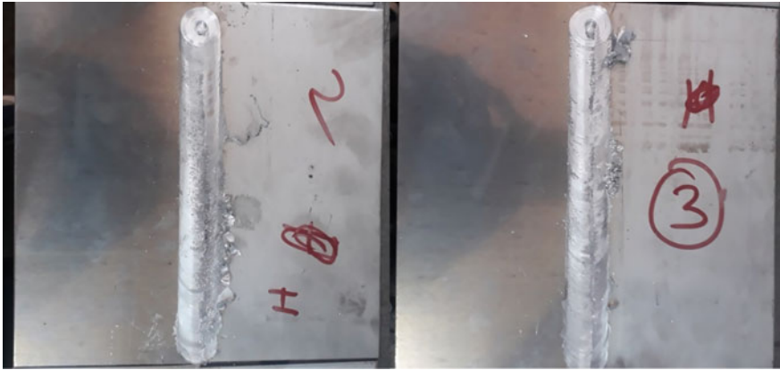
Fig. 3 Fabricated welded joint by using of hexagonal and squared structured profiles, respectively
