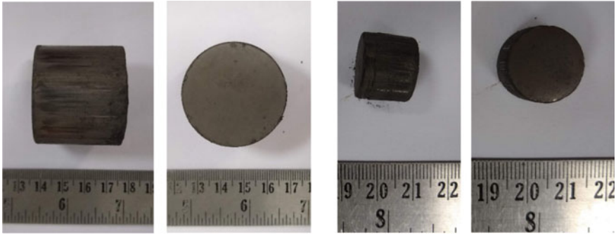
Fig. 3 Green compacts (40 mm diameter on left and 16 mm diameter on right)
