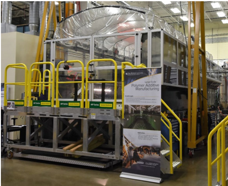
Fig. 2 Big Area Additive Manufacturing (BAAM) [46]
