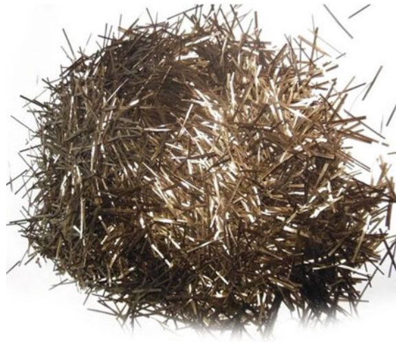
Fig. 2 Chopped silicized/silane treated basalt fiber for reinforcement (1 mm diameter and 3 mm length)
