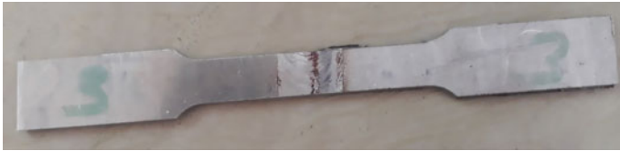
Fig. 5 Tensile specimen prepared by using the squared profiled tool
