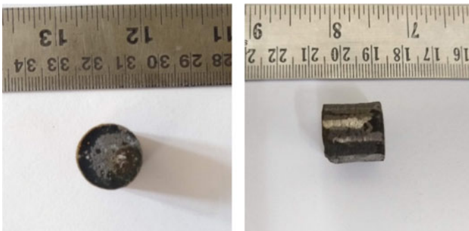
Fig. 14: 20 mm diameter consolidates of same alloy composition powder made using tungsten carbide ball and vial
