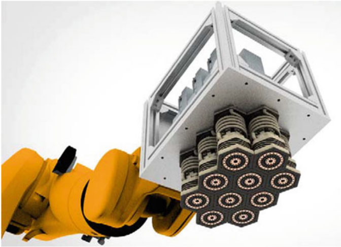
Fig. 1 Drape gripper with hexagonal pixels [21]
