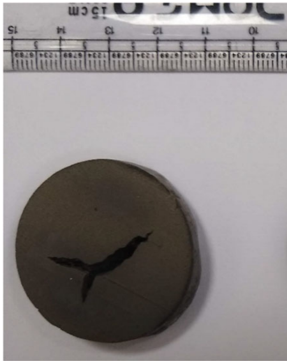
Fig. 7 EDM cut consolidate sections for further testing
