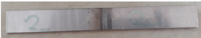
Fig. 8 Flexural welded specimens—hexagonal profile
