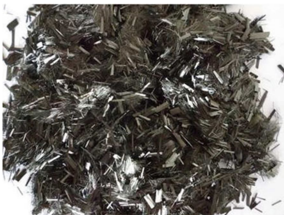
Fig. 3 Raw black chopped carbon fiber (3 mm length) with 95% carbon content
