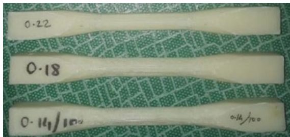
Fig. 3 ABS specimen with a different layer thickness (without acetone treatment)
