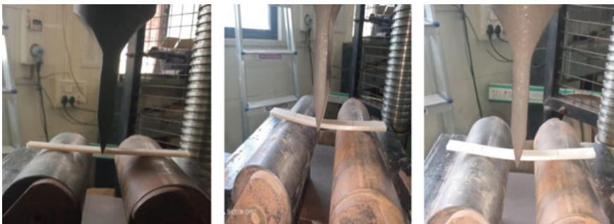
Fig. 11 Flexural testing of 3D printed composites
