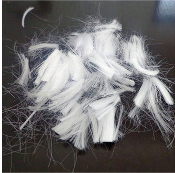
Fig. 1 Chopped cellulose fiber strands (250 \mu\text{m} diameter)
