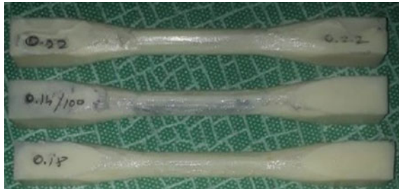
Fig. 2 ABS specimen with different layer thickness acetone treatment
