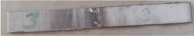
Fig. 9 Flexural welded specimens—squared profile
