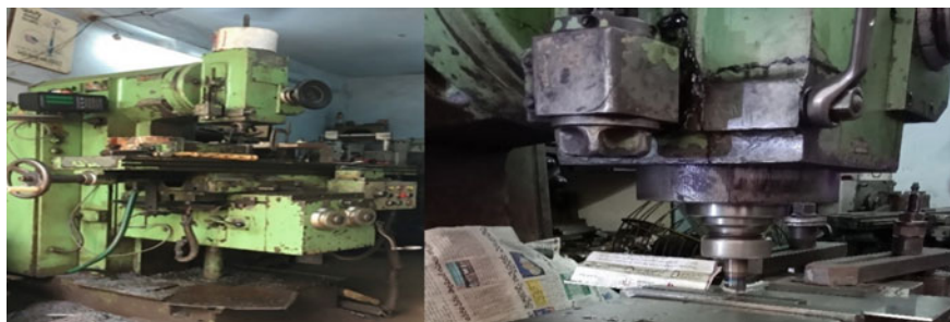
Fig. 1 Friction stir welding setup
