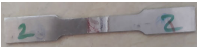
Fig. 4 Tensile specimen fabricated by using the hexagonal profiled tool
