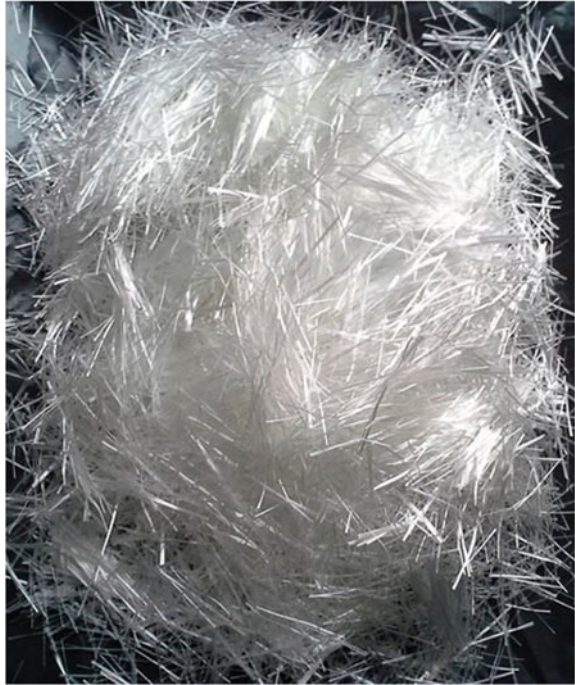
Fig. 4 Raw plain chopped glass fiber (10 \mu\text{m} diameter and 3 mm length)
