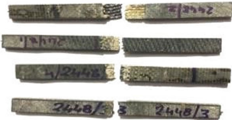
Fig. 8 Fractured specimens of flexural test
