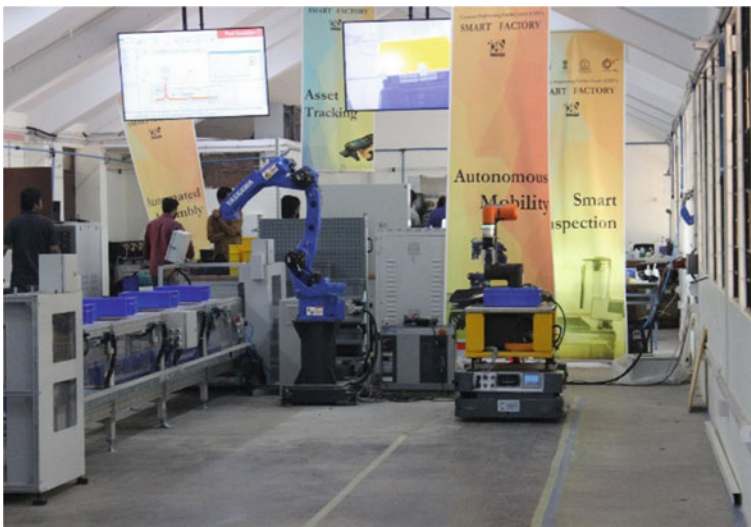
Fig. 18 The experimental test bed available with collaborative manipulator robot and industrial robot present at the CEFC, IISc Bangalore
