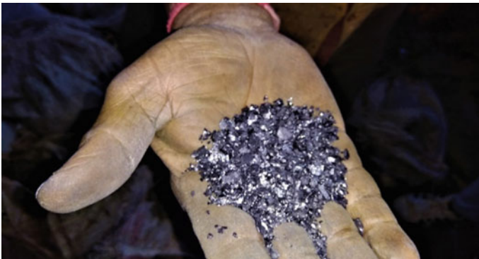
Fig. 3 Ferro silicon magnesium (nodulariser)
