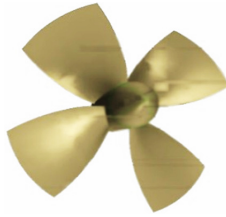
Fig. 2. Propulsive propeller of the ROV
