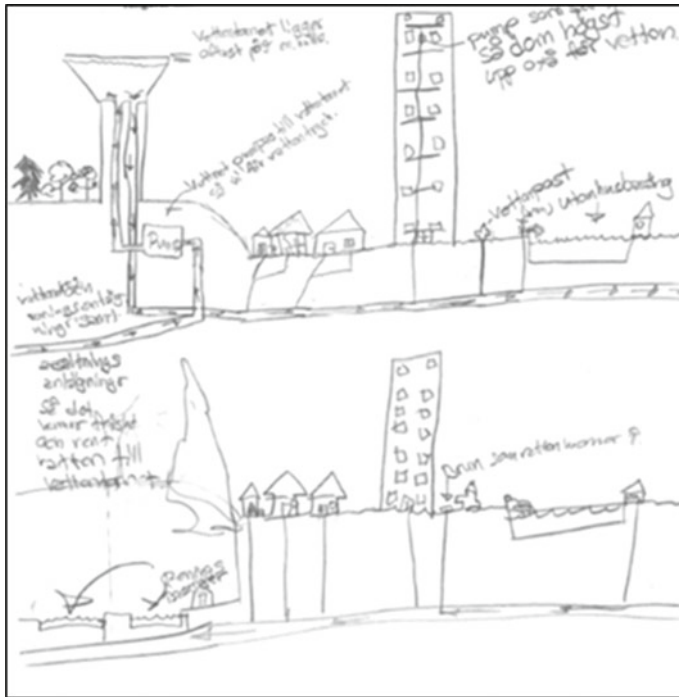
Fig. 11.6 Example of a system drawing showing the visible components as well as the pipe networks under-ground
