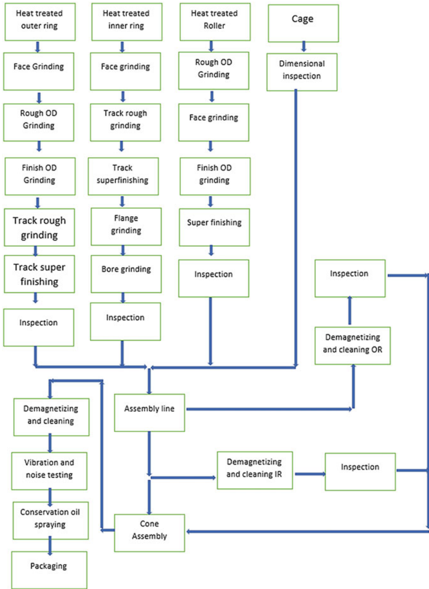
Fig. 1 Manufacturing process sequence in the fabrication shop
