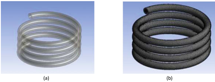
Fig. 1 a Four-turn helical heat exchanger model. b Four-turn meshed helical model
