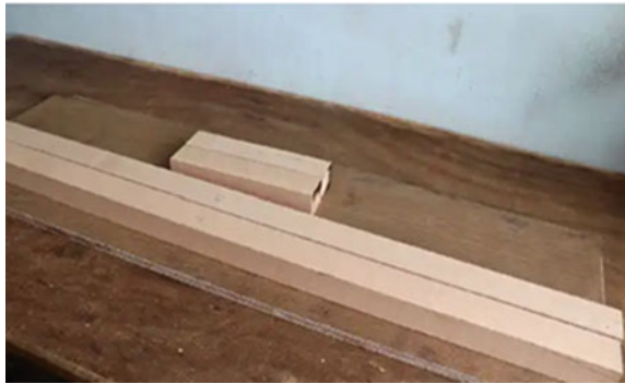
Fig. 3 Plywood and wooden blocks used in making a mini lathe
