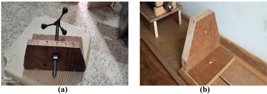
Fig. 6 Preparation of tailstock: a assemblage of tailstock components and b placement of the tailstock on the prepared slot
