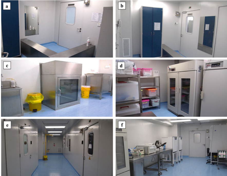
Fig. 3.3 cGMP Facility in Centre for Tissue Engineering and Regenerative Medicine (CTERM), Faculty of Medicine, Universiti Kebangsaan Malaysia (UKM). (a) Cleanroom grade B area is equipped with various equipment for cell manipulation; (b) Grade C corridor; (c) Grade D change room for change street cloth to scrub; (d) Waste disposal via waste hatch; (e) Production personnel working in cleanroom grade B
