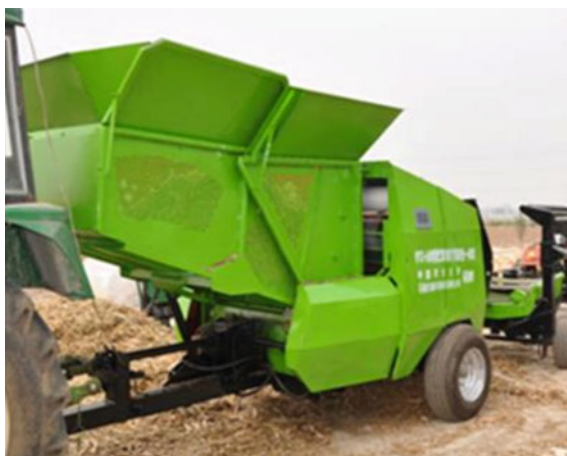
Fig. 10.34 SMR1000H green fodder harvester and baler
