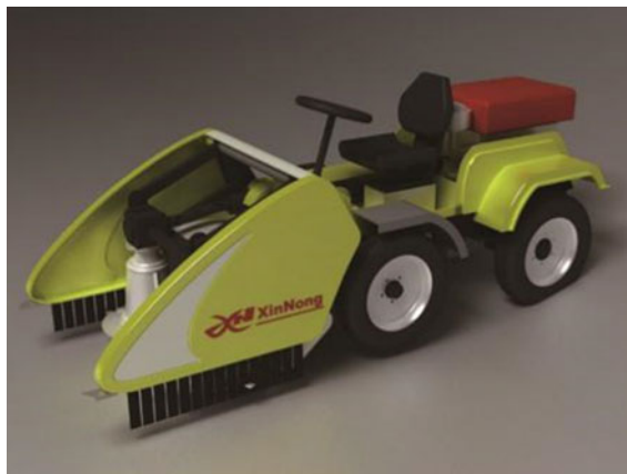
Fig. 10.24 22.4-3 self-propelled cutting and conditioning machine. 1. runner; 2. cutter; 3. cutter head; 4. roller; 5. upper connecting rod; 6. floating spring; 7. bracket; 8. frame; 9. lower connecting rod; 10. hydraulic cylinder; 11. hydraulic cylinder base; 12. crushing roller
