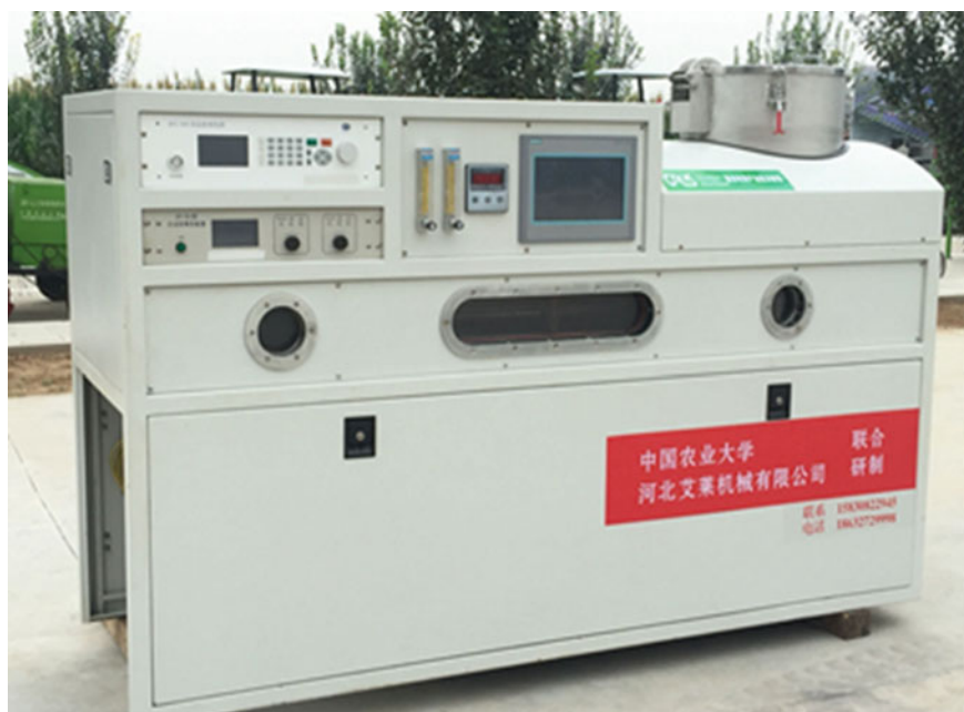
Fig. 10.8 Cold plasma seed treatment equipment
