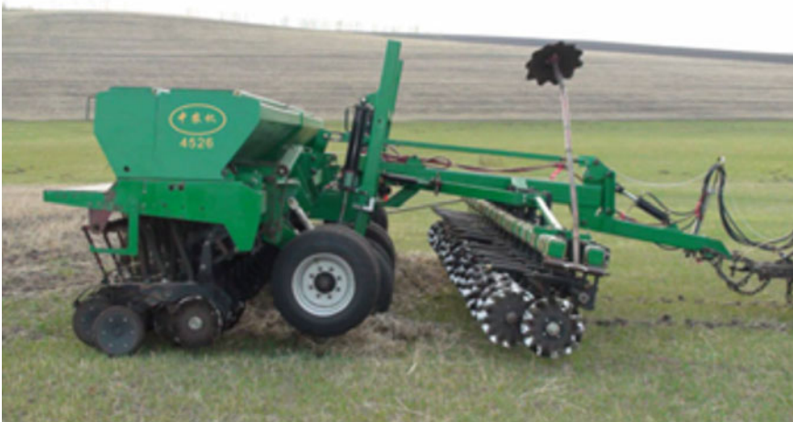
Fig. 10.13 2BF-3620 no-tillage planter
