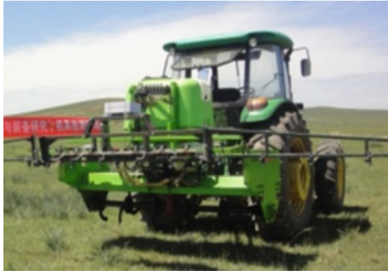
Fig. 10.12 9QPY-2.2 Stellera chamaejasme weeding machine
