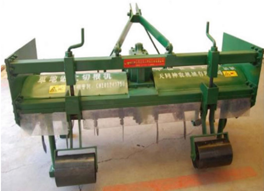
Fig. 10.14 9QP-830 grass root cutter
