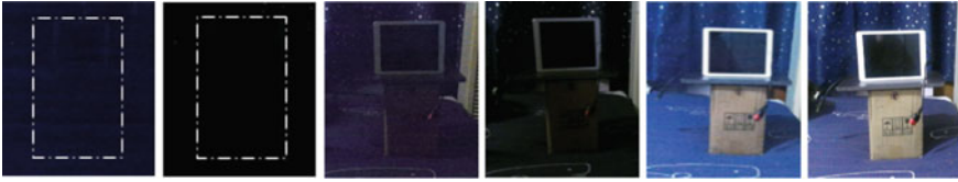
Fig. 2 In the figure above, from left to right are data from Azure Kinect in dark environment, data from Kinect 2.0 in dark environment, data from Azure Kinect under 20 W lamp, data from Kinect 2.0 under 20 W lamp, data from Azure Kinect under 60 W lamp, data from Kinect 2.0 under 60 W lamp. The dashed box indicates the test object
