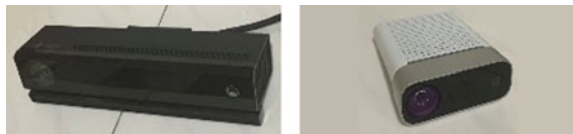
Fig. 1 Two generations of Kinect (Kinect 2.0 on the left and Azure Kinect on the right)
