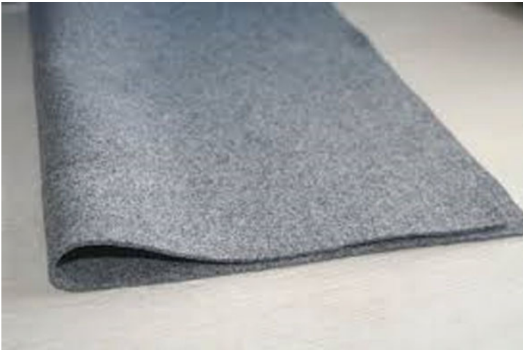
Fig. 3 Geosynthetic used for present study
