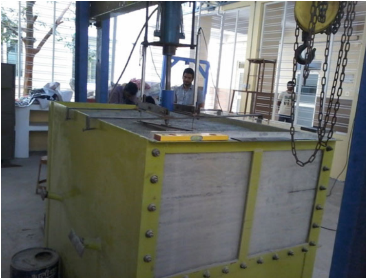
Fig. 5 Load-settlement test on square footing
