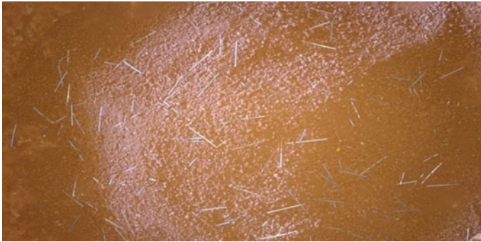
Fig. 5 Randomly distributed fibers mixed in the soil
