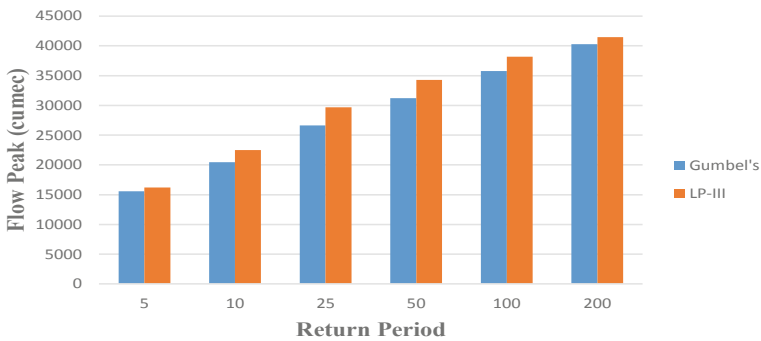
Fig. 7 Comparison of flows computed using Gumbel's extreme value distribution and Log-Pearson type-III distribution
