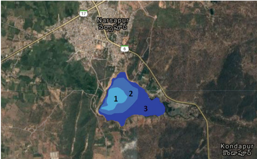
Fig. 5 Water spread area in different time periods. Note 1: Min. water spread area observed from Sentinel-1 SAR data on 22-Aug-2020. 2: water spread area observed from SRTM DEM. 3: Max. water spread area observed from Sentinel-1 SAR data on 21-Oct-2020
