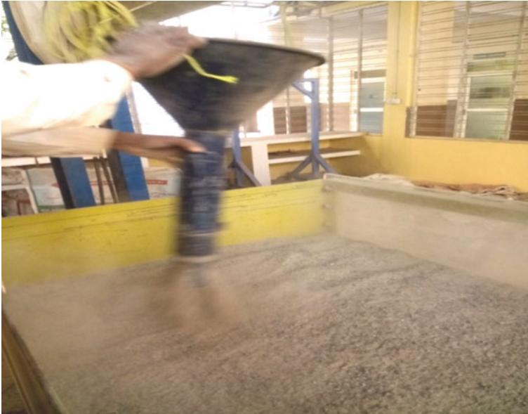
Fig. 4 Filling tank by sand rain technique
