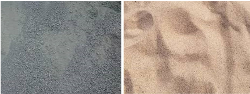
Fig. 2 Crusher dust and sand used as foundation material
