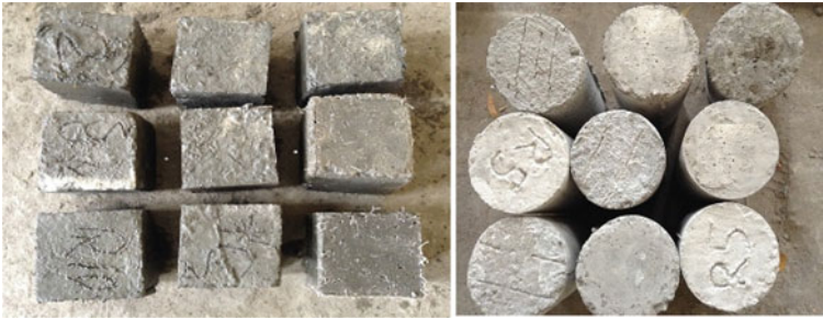
Fig. 2 Specimens of PC and PPFRC (12 and 20 mm)
