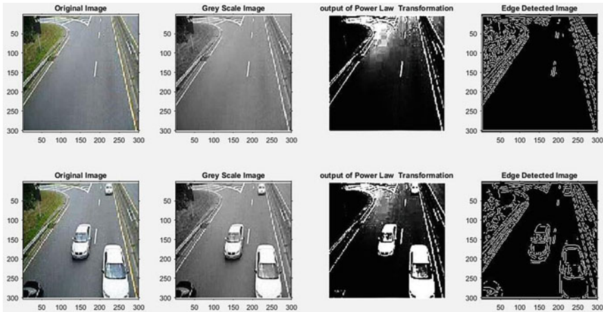
Fig. 14 Output of edge detection technique
