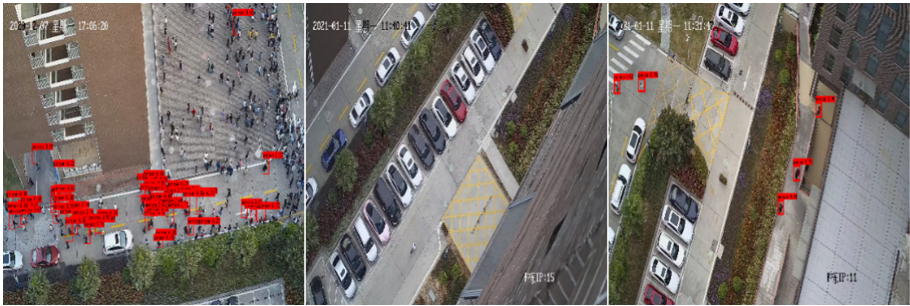
Fig. 5. The high-altitude pedestrian detection results of YOLOv3 [10].
