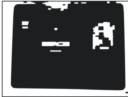
Fig. 5. Image thresholding result of the first projector's gradient image.
