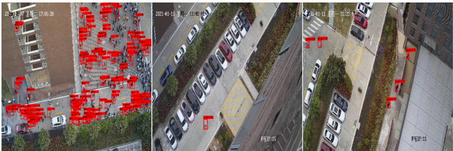
Fig. 6. The high-altitude pedestrian detection results of the YOLOv3-M.
