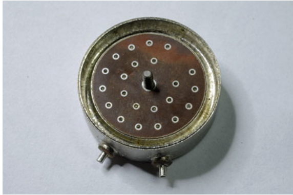
Fig. 10.8 First Cochlear feedthrough with titanium flange before welding to the titanium case that housed the electronic circuitry (Image copyright David Cowdery, supplied courtesy of David Cowdery)
