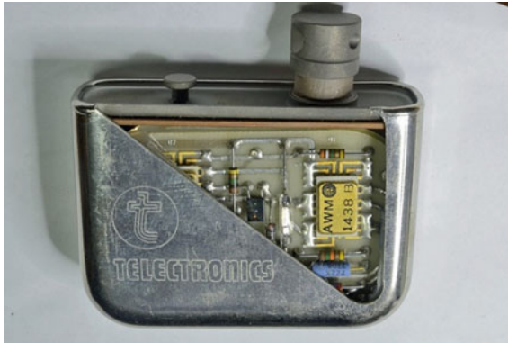
Fig. 10.5 A later model Teletronics pacemaker (circa 1976) with a bare terminal assembly identical to that used on the first P10 (Image copyright David Cowdery, supplied courtesy of David Cowdery)
