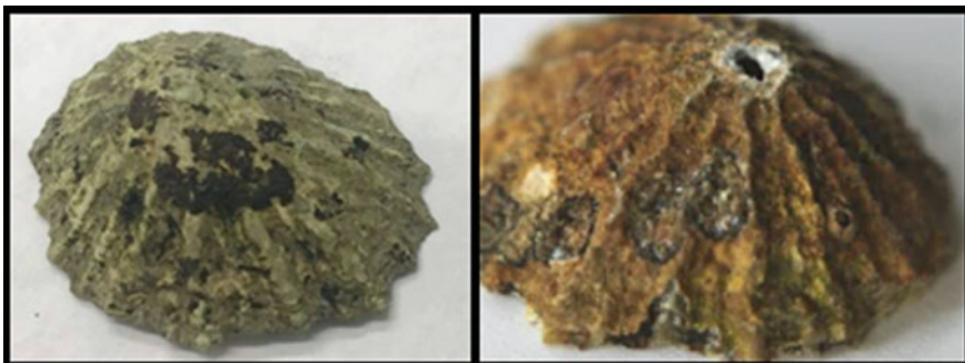
Fig. 3.8 An intact limpet shell (left) and shell of a limpet after an impact test (right) [48] (Modified and adapted with permission from)
