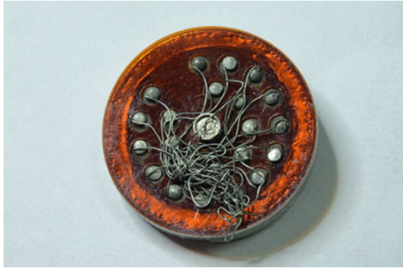
Fig. 10.9 The electrode side of the first Cochlear feedthrough with polyimide insulator and parylene-coated platinum electrode wires soldered into the platinum tubes (Image copyright David Cowdery, supplied courtesy of David Cowdery)
