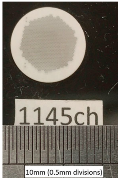
Fig. 10.12 Co-fired alumina-platinum feedthrough with the record-breaking 1145 electrodes [32]. This was achieved in a diameter of just 7 mm, as shown by the millimeter scale (Image copyright Andrew Ruys, supplied courtesy of Andrew Ruys)
