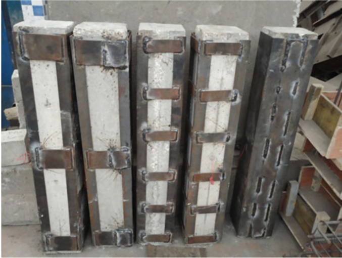
Fig. 3 Strengthened RC column with steel jackets with 3 battens, 6 battens, and complete steel plating [13]
