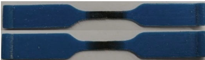
Fig. 14 Build fatigue samples showing a stepwise gradient (top) and a continuous gradient (bottom) in the material gradient transition region [63]
