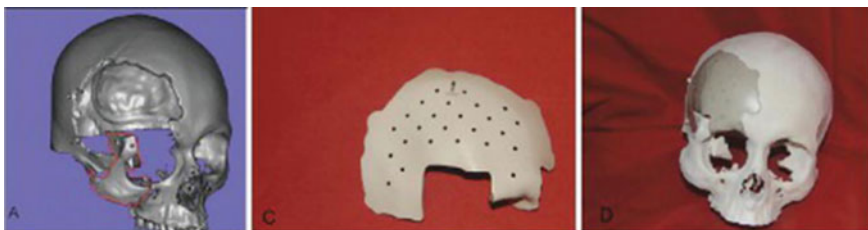
Fig. 7 a Skull defect using CAD model, c cranial implant SLA fabrication and d an implant placed into skull model, (reprinted with permission from [37])
