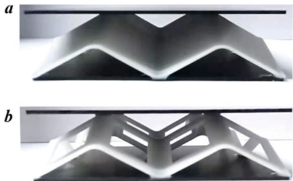
Fig. 2 3D printed spherical-roof contoured-core designs: a common SRCC design; b novel SRCC design with four diamond-shaped notches
