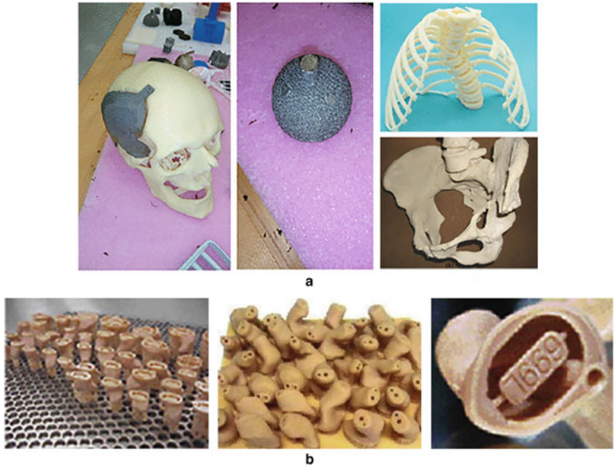
Fig. 11 a Medical applications—AM (Reprinted with permission from [58]), b individually customized mass-produced hearing aid shells (Reprinted with permission [59])
