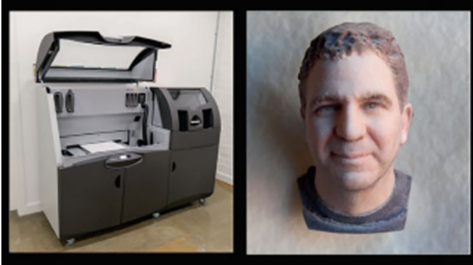
Fig. 5 Color binder's human portrait in 3D and PBP machine on the left, (reprinted with permission from [15])
