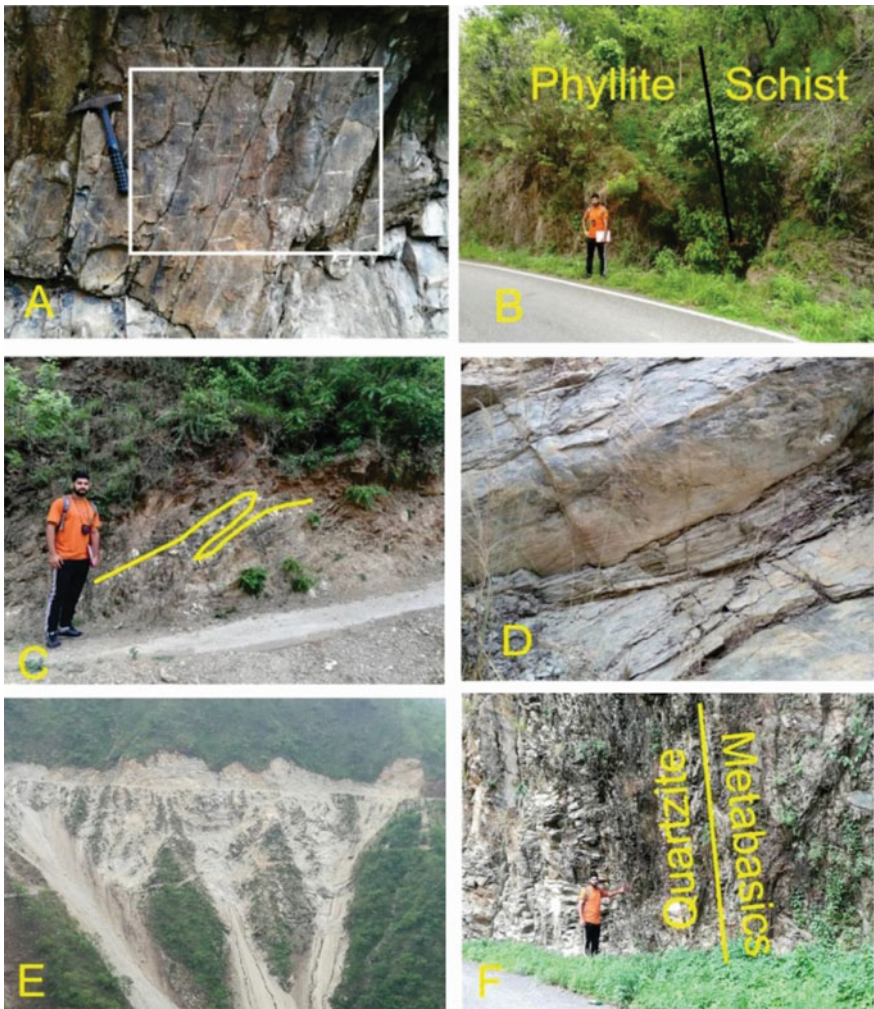
Fig. 8.6 Showing a jointed and fractured quartzite with quartz veins; b lithocontact with sheared material and seasonal nala is flowing along contact; c refolded crushed quartz vein in sheared and crushed phyllite suggesting tectonic influence; d crushed phyllite in margin of fold crest quartzite; e folding seen from afar along newly road-cut section near fault zone; and f closely placed lithocontact with a few meters of shear zone
