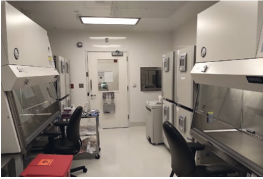
Fig. 3.2 Image of one of six Good Manufacturing Practice (GMP) laboratories inside the GMP facility at the University of California Davis, Institute for Regenerative Cures. This is where CD34+ stem cells and progenitor cells are isolated for clinical trials. It is an ISO7 (Class 10,000) cleanroom laboratory with temperature, air pressure, and humidity control. This assures a tightly controlled and highly reproducible environment avoiding contamination by air particulates. Any person entering this area must undergo a special gowning procedure and have special training pertaining to procedures applied in GMP laboratories (courtesy of Professor Gerhard Bauer, Director of GMP laboratory)
