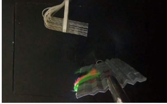
Fig. 9 Flow reversal for corrugated wing at AOA +18° and Re_c 120,000
