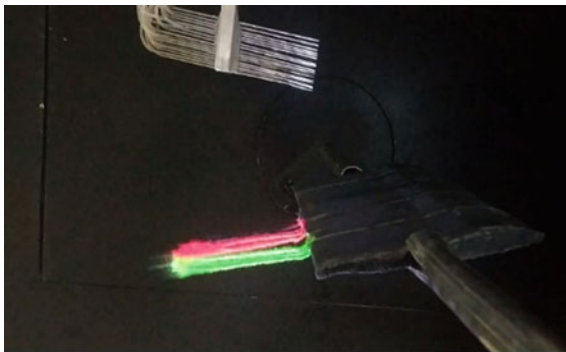
Fig. 6 Tuft flow visualization for hybrid wing at AOA +20^\circ and Re_c 46,000
