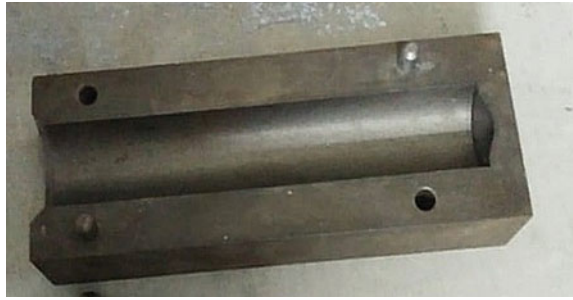
Fig. 6 Cylindrical rod mold to form as casted Al-MMC rod
