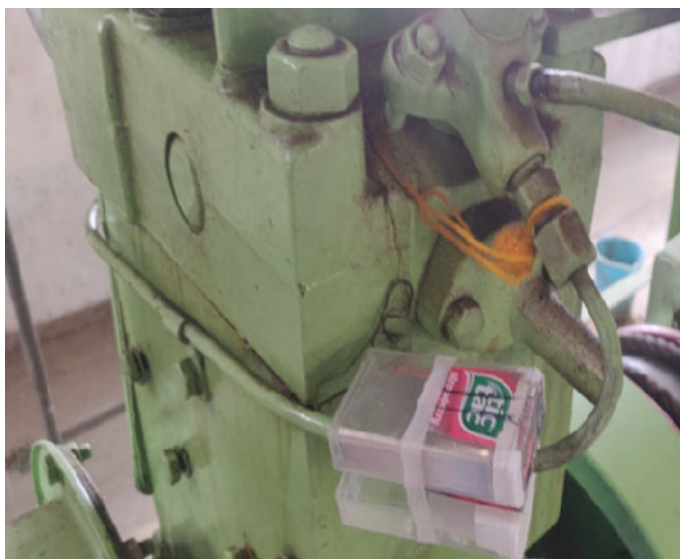
Fig. 1 Photograph of Neodymium N52 Magnets fixed on diesel engine fuel line
