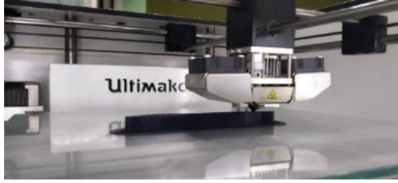
Fig. 3 3D printing of corrugated wings using a Ultimaker S3 3D printer
