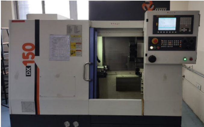
Fig. 10 CNC lathe machine used for turning of Al-MMC
