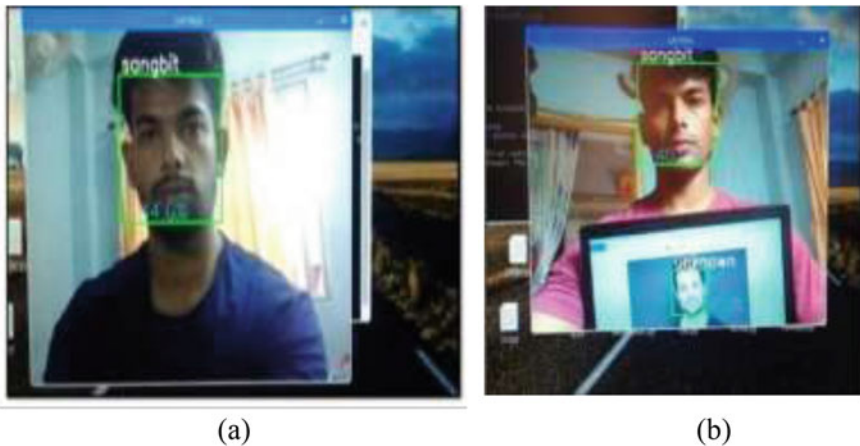
Fig. 6 Real-time face recognition a successful detection and b unknown detection
