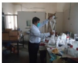
(b): Experimental set up of CO 2 gas preparation
