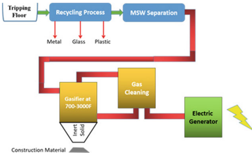
Fig. 2 Schematic diagram of electricity generation by gasification
