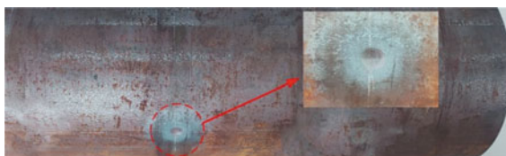
Fig 5.8 Gouge specimen of pipeline
