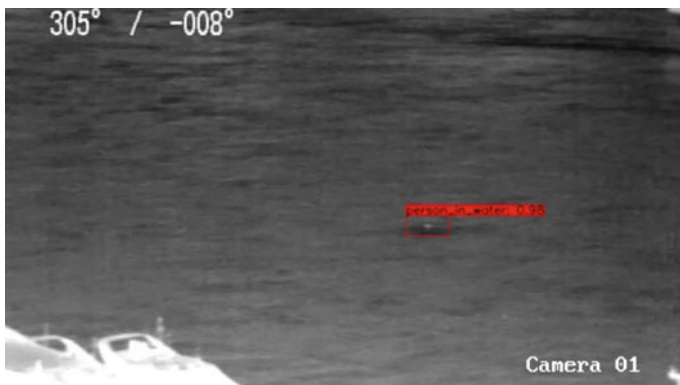
Fig. 29.10 Detection results of people falling into the water under thermal imaging mode (depression angle 8^\circ )
