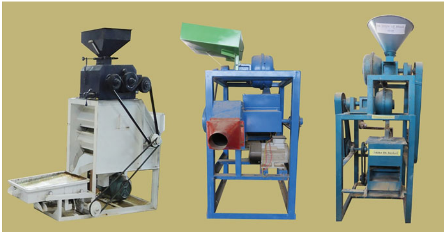
Fig. 15.3 Rubber roll sheller type, single-stage and double-stage centrifugal type millet dehusker (from left to right)
