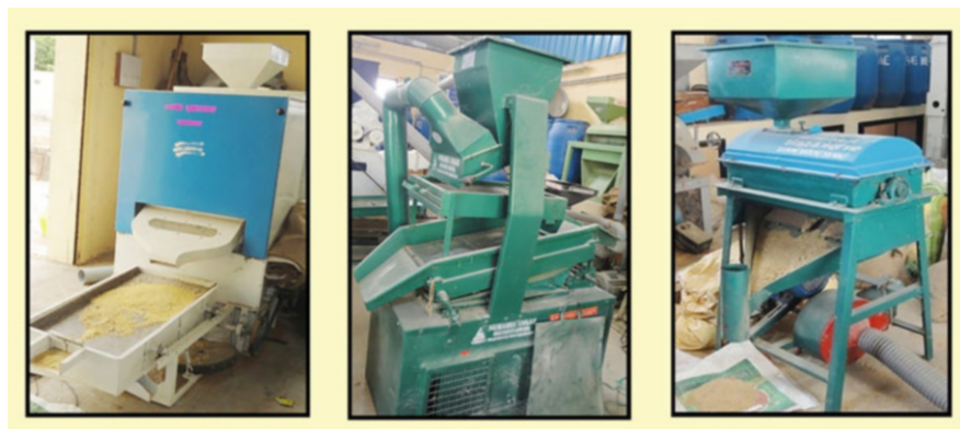
Fig. 15.4 Cleaner cum grader, destoner and pearler (from left to right) for millet processing
