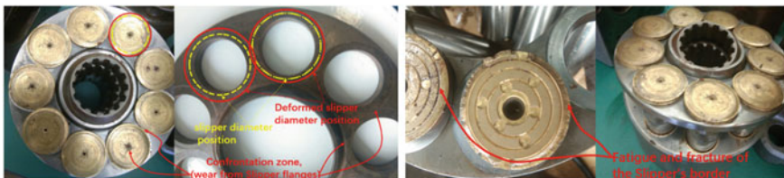
Fig. 2 Large elastic deformation, wear and fracture of the slipper and retainer
