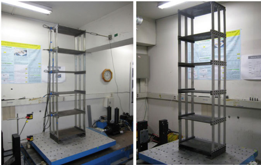
Fig. 2 Experimental configuration of a five-story shear frame [31]
