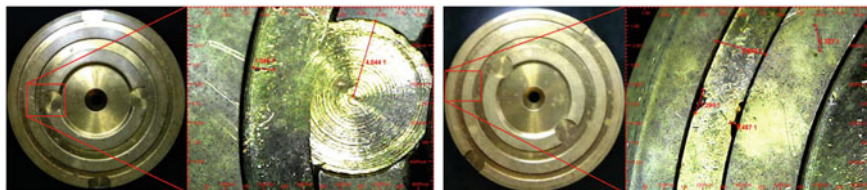
Fig. 7 The surface of the slipper pad after the test
