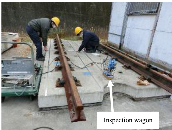
Fig. 11 Local vibration testing on the railway track slab
