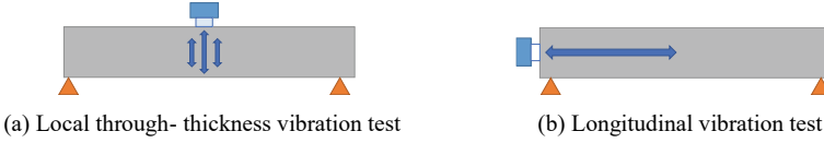
Fig. 2 Schematic diagram of (a) local through-thickness vibration test and (b) longitudinal vibration test
