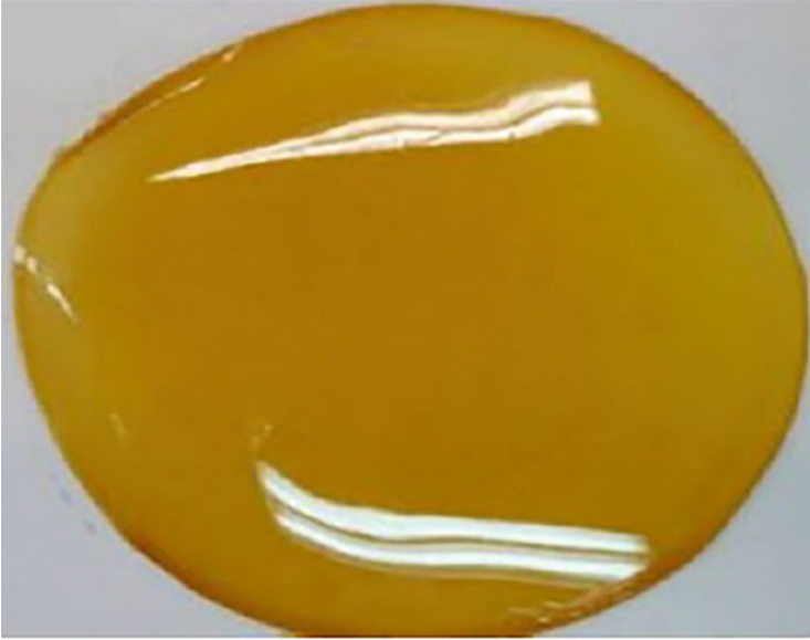
Fig. 4.5 Bilayer film of isolated protein from hake and zein (Source: Nogueira and Martins et al. (2018))
