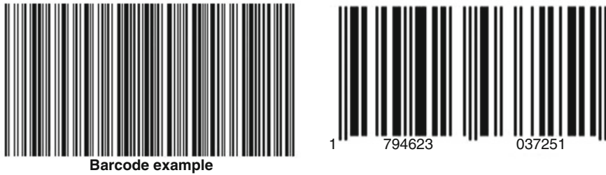
Fig. 6.7 An example of a Code-128 barcode (left) and EAN-13 code (right) (Source: generated at https://www.cognex.com/resources/interactive-tools/free-barcode-generator )
