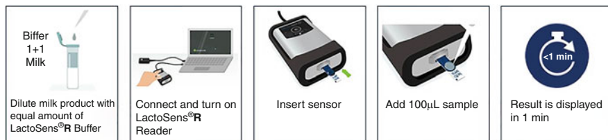
Fig. 6.12 LactoSens® operating procedure step-by-step (Source: Image provided by DirectSens (2021))
