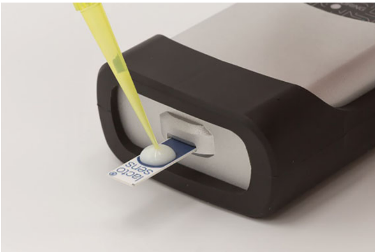
Fig. 6.10 LactoSens ® biosensor assay kit for lactose detection in dairy products (Source: Image provided by DirectSens (2021))
