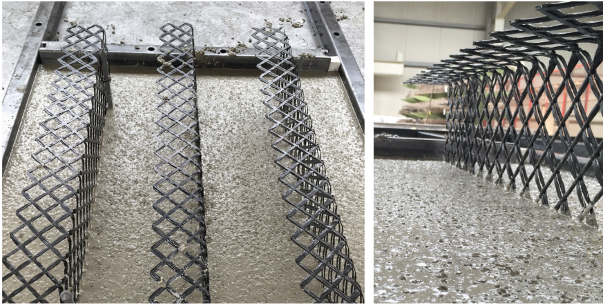
Fig. 3 Pre-formed mesh reinforcement
