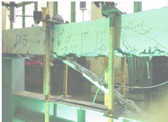
Fig. 7 Typical failure mode of the CFRP strengthened beams
