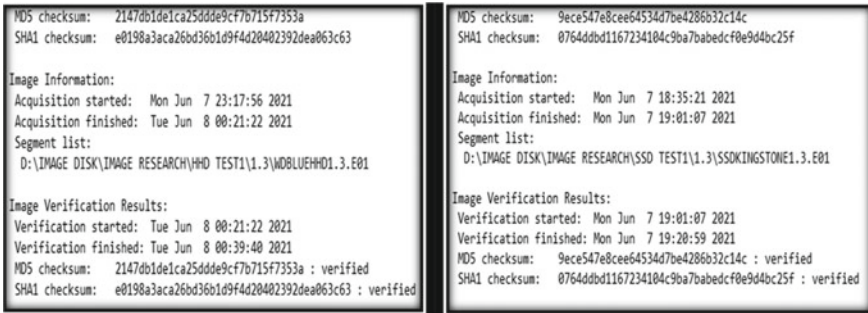
Fig. 8 Sample FTK-acquired images properties for HDD (left) and SSD (right) (full format scenario)
