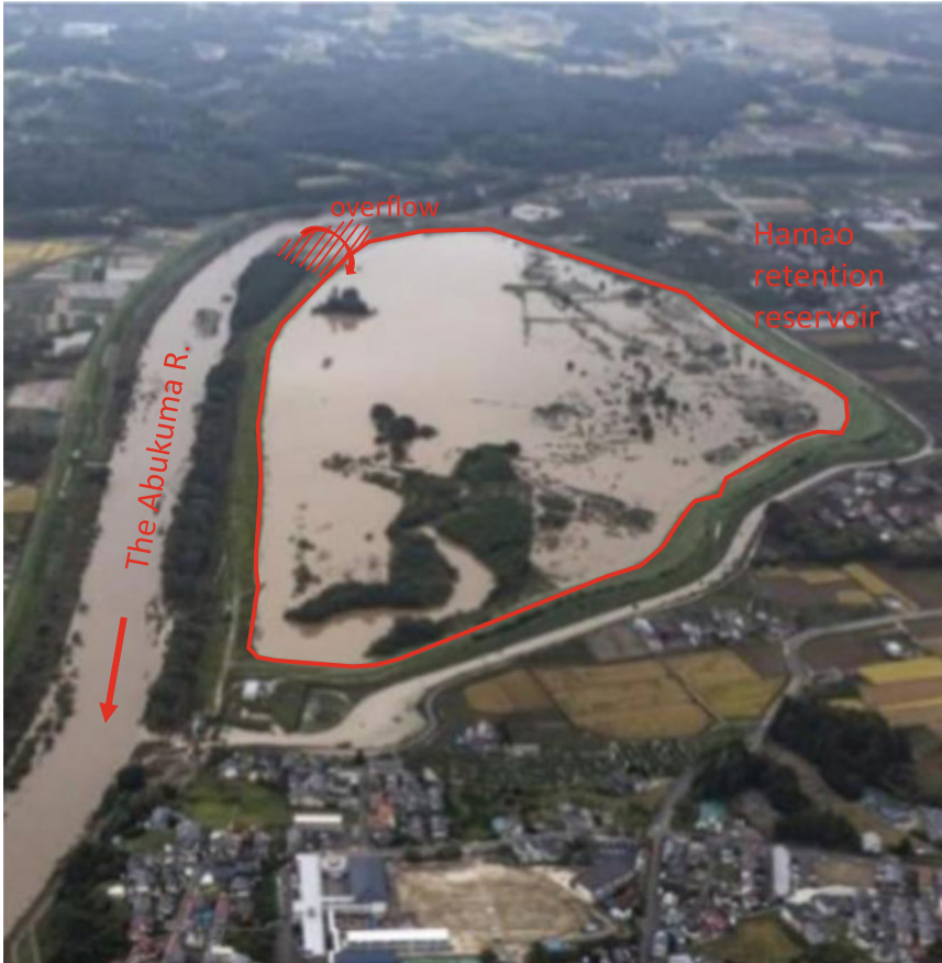
Fig. 14.5 Pooling the flood water successfully (2.6 million square meters) at Hamao Retention Reservoir (modified from MLIT 2012)
