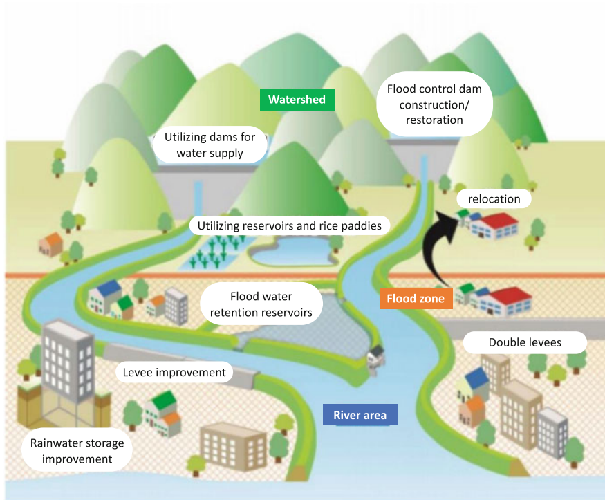
Fig. 14.8 Overall image of basin-wide flood management project (source: MLIT, 2021)
