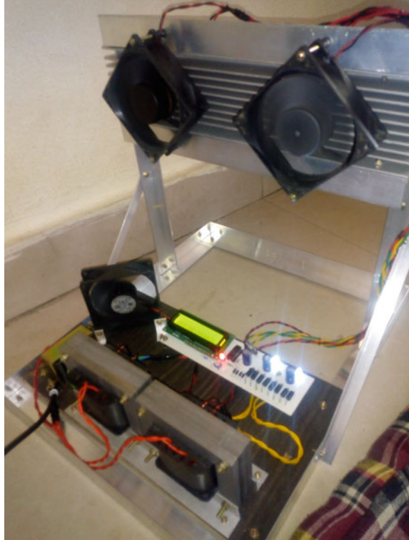
Fig. 5 Hardware implementation of atmospheric water generator
