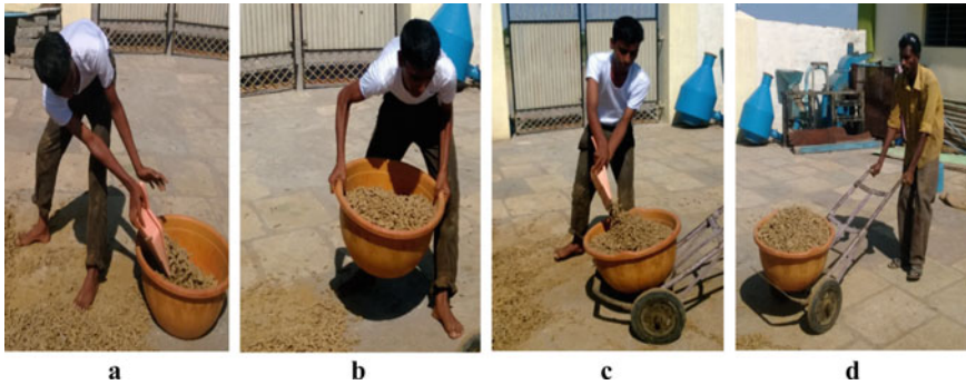
Fig. 5 Postures adapted by workers (a) and (b), ergonomic intervention (c) and (d)
