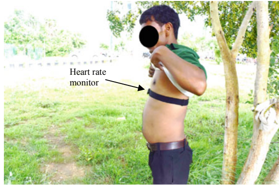
Fig. 1 Chest strap type heart rate monitor attached to the worker
