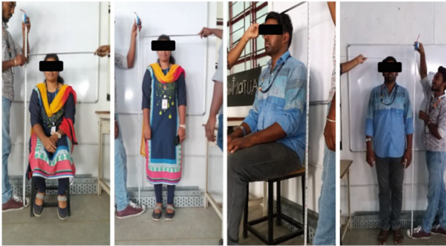
Fig. 5 5th Percentile female sitting and standing height and 95th Percentile Male sitting and standing height
