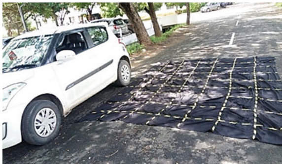
Fig. 9 Blind spot measurement for Vehicle A
