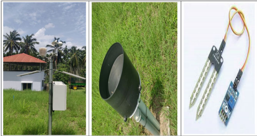
Fig. 2 Automatic Weather Station, Rain guage and soil moisture meter installed at the farmer’s field in Sethumadai village as a critical infrastructure to minimize risks due to weather vagaries
