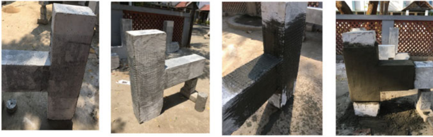
Fig. 4 Process of retrofitting the beam-column joint specimen
