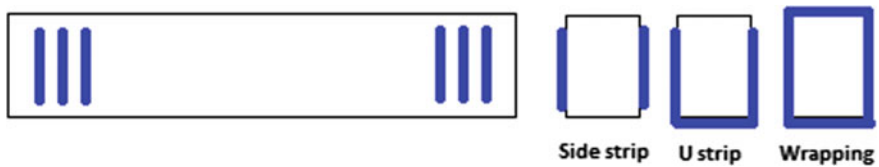
Fig. 4 FRP strips strengthening of RCC beam in shear zone
