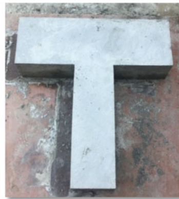
(b) Exterior beam-column joint specimen
