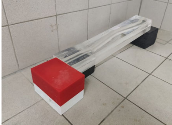
Fig. 5 Assembly of scaled-down penstock model
