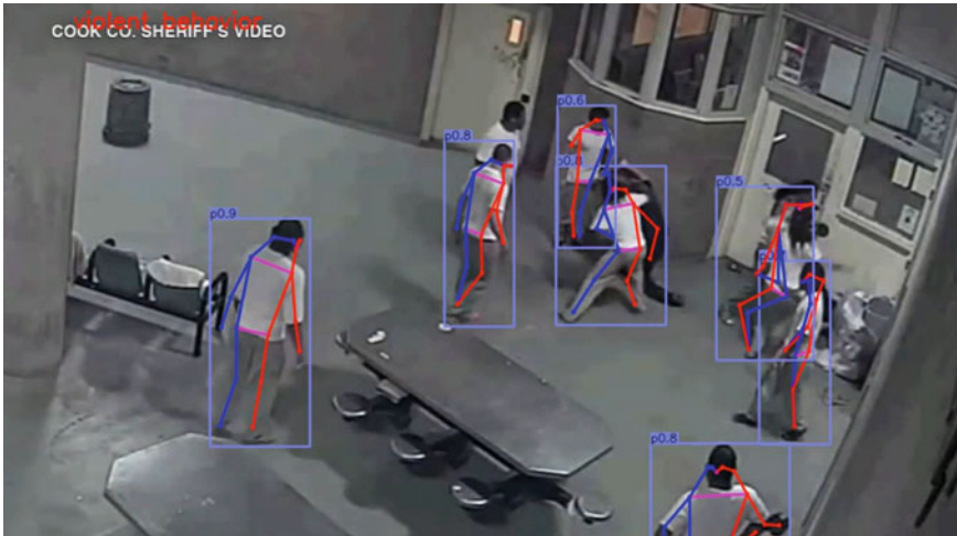
Fig. 4 Violent behavior recognition and pose estimation visualization
