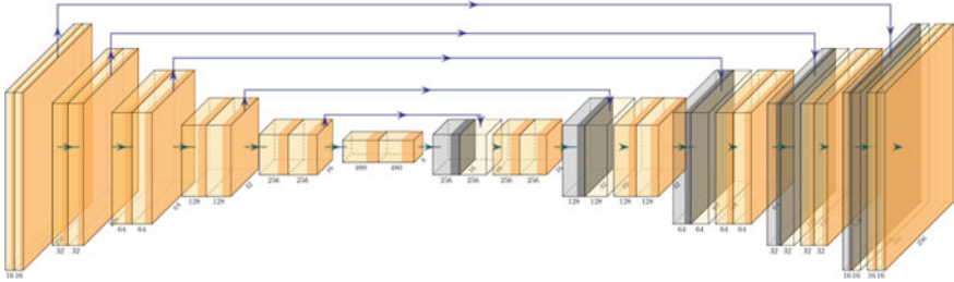
Fig. 2 The network structure of generic nnU-Net
