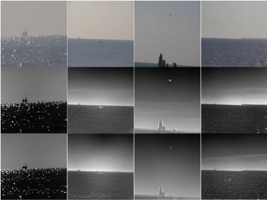
Fig. 5 Display of infrared image translated from visible image (The second line of infrared image is generated by the proposed method, and the third line of infrared image is generated by CycleGAN)
