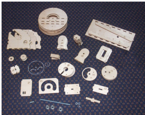
Fig. 11 Components of pan tilt mechanism
