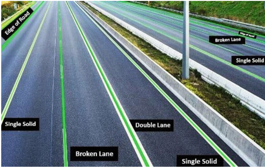
Fig. 9 A road network lines annotated using the Lines and Spline annotation method
