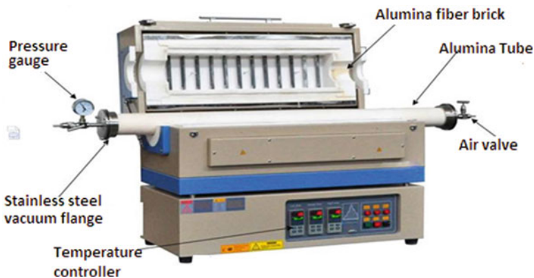
Fig. 6 High-temperature tubular furnace and its different subassemblies Kept in Material testing laboratory in IIT, Roorkee
