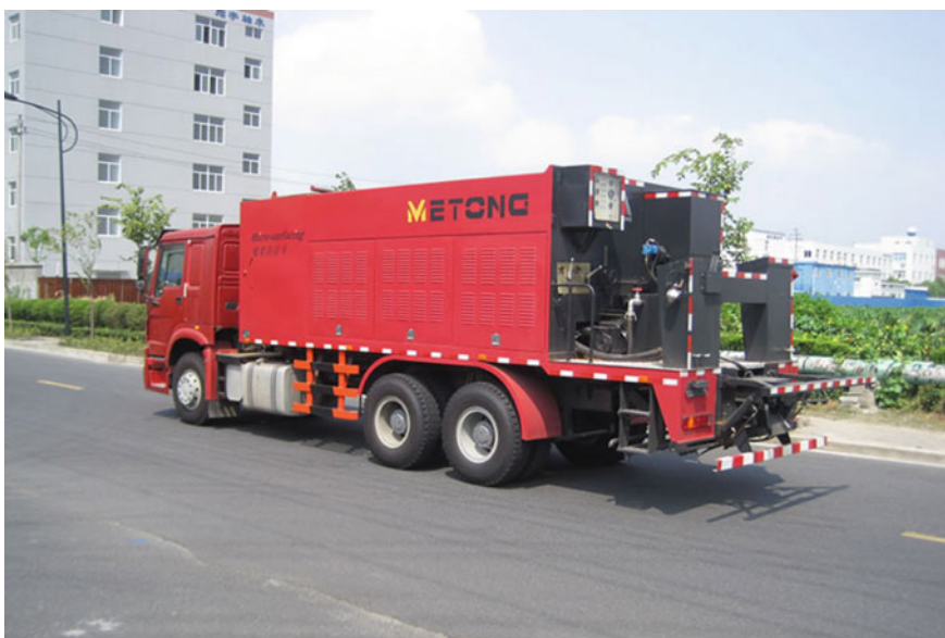
Fig. 8 Microsurfacing machine LMT5255TXF
