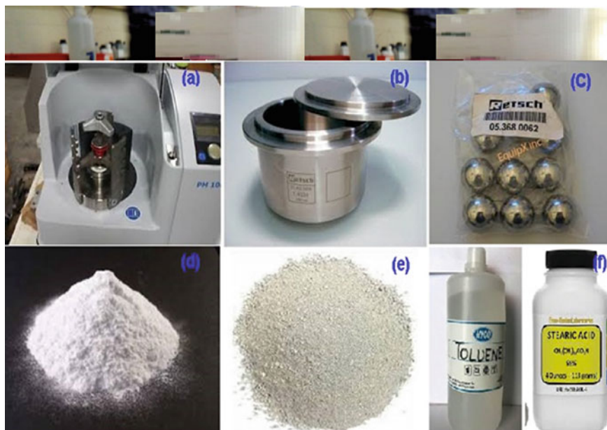
Fig. 4 Initially all the materials required for the experiment were made ready in the Material testing laboratory a) Retsch PM100 Ball Mill used for mixing as well as milling, b) Hard stainless-steel jar used to hold hard steel ball that helps/milled the material under processes, c) Hard stainless-steel ball that is used with Jar d) ceramics powder, i.e. \text{Al}_2\text{O}_3 , e) Aluminium powder used here as a base material for composite f) Liquid toluene is used as a solvent and Stearic acid is used as lubricant in the material preparation method
