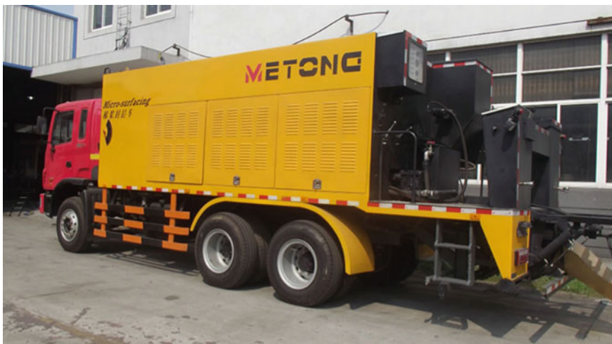
Fig. 7 Microsurfacing machine LMT5256TXF [10]
