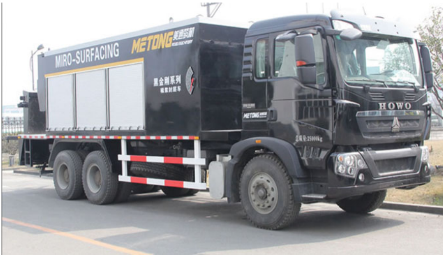
Fig. 6 Microsurfacing machine LMT5310TXF [9]
