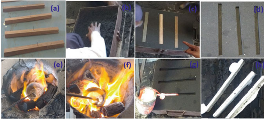
Fig. 2 a) Wooden patterns used for open casting, b) Preparation of green sand for casting, c) Patterns are placed to produce mould cavity, d) Mould cavity is ready for pouring liquid metal, e) and f) Aluminium is melted in an open furnace, g) Liquid metal is poured into the cavity and h) Casting of aluminium is ready for different samples for test
