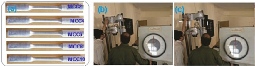
Fig. 10 a Five different test samples used for tensile test, b Initial setting of sample in UTM has been done and c shows the final elongation of the sample
