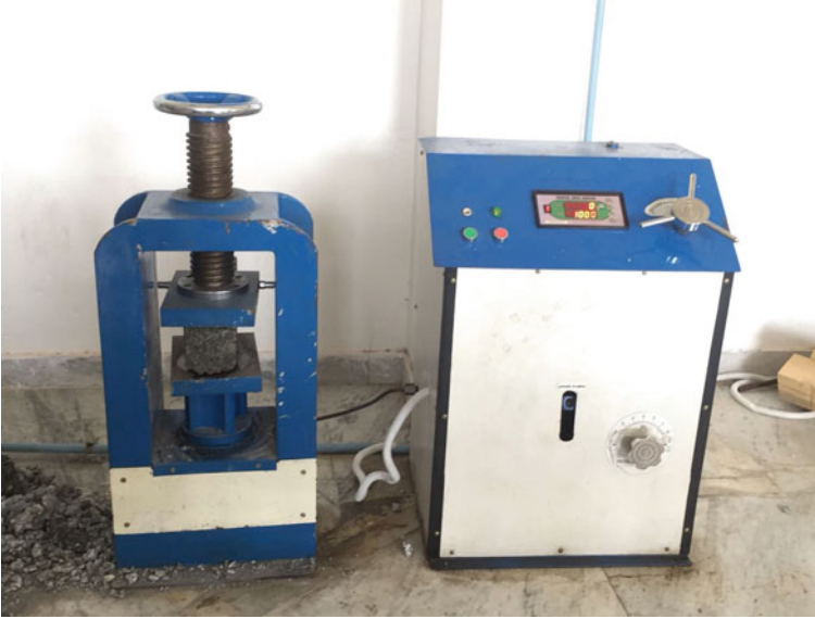
Fig. 2 Compressive strength test
