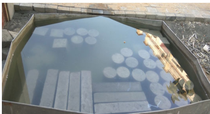
Fig. 1 Curing of concrete samples
