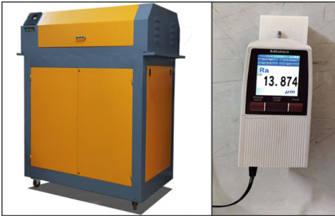
Fig. 4 Jak Machinery JM1200 FDM type 3D printer and Mitutoyo SJ 210 surface roughness tester respectively
