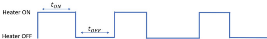
Fig. 4 Digital variable frequency pulse signal
