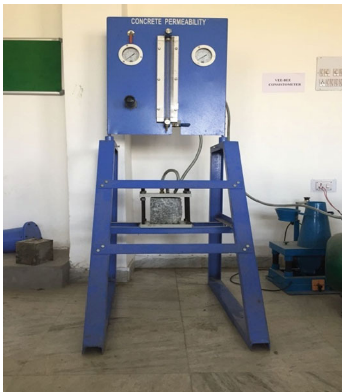
Fig. 3 Water permeability test
