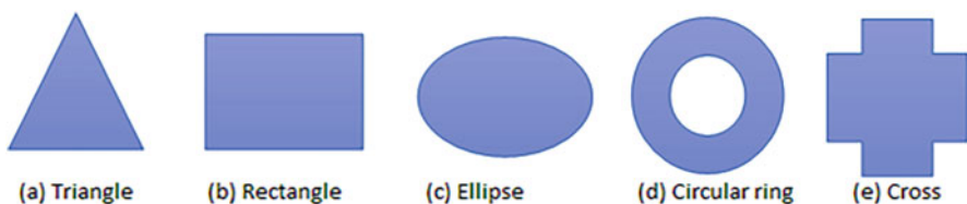
Fig. 13.2 Various shapes of the patch antenna
