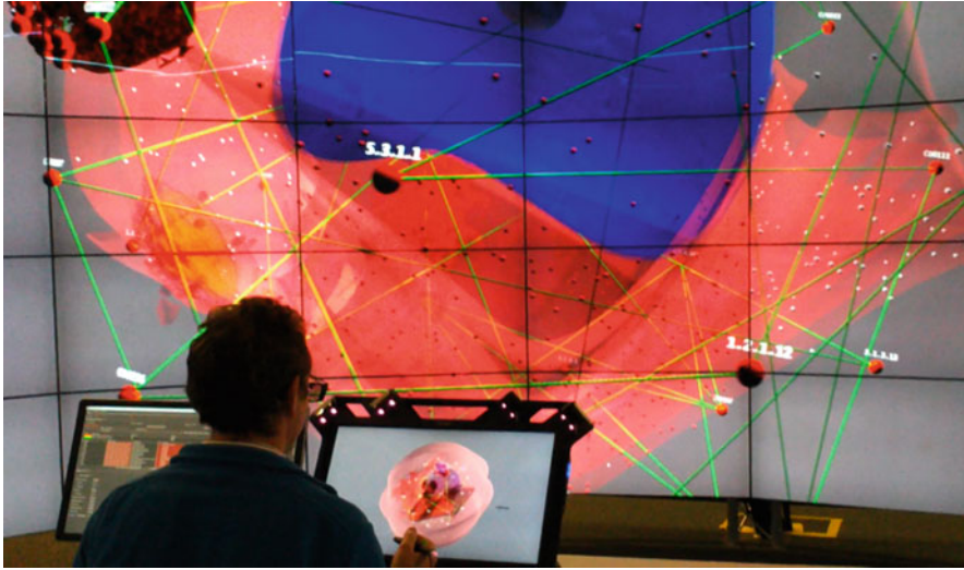
Fig. 12.13 Exploration of metabolic pathways within the spatial context using an immersive environment based on CAVE2 (stereoscopic 3D) and zSpace (stereoscopic fishtank 3D) (from Sommer and Schreiber (2017b))
