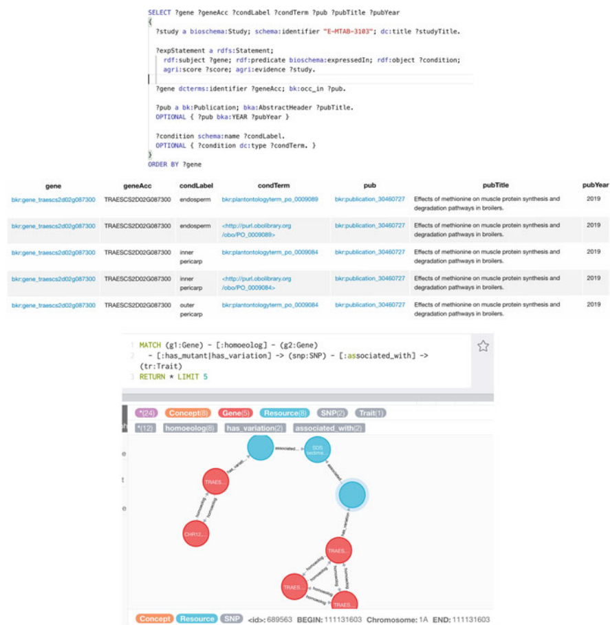
Fig. 8.3 Querying and using graph data. Top: a SPARQL example, the Semantic Web standard to query RDF data, based on a graph pattern syntax (e.g., ?study matches any study node having an identifier and a title). The query matches data that were integrated from both KnetMiner and EBI GXA (middle). Bottom: a simplified case of the Cypher queries (the Neo4j query language for property graphs) that KnetMiner uses to relate a gene to relevant entities, which is at the basis of application results described in Sect. 8.2
