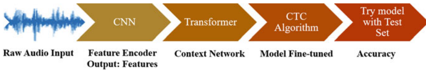
Fig. 1 System model workflow from input; training steps and generating accuracy based on test set
