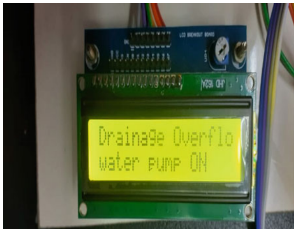
Fig. 11 Overflow alert on LCD
