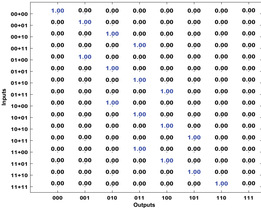
Fig. 11 Experimental results of two-qubit adder on IBM quantum device: IBM QASM (32 qubits) [10]
