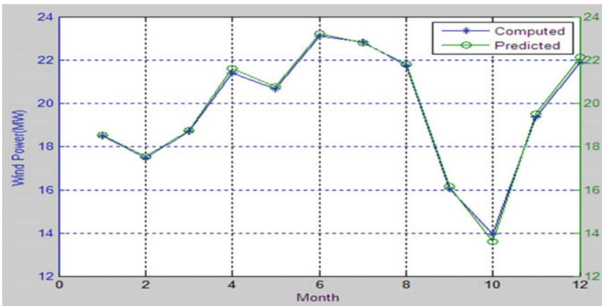
Fig. 14 Predicted values of wind power in comparison with computed power with ANN
