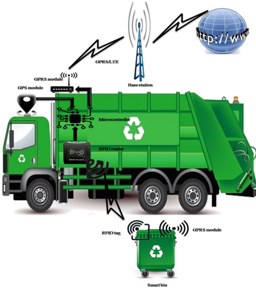
Fig. 2 Communication link between on board devices of smart truck and bin
