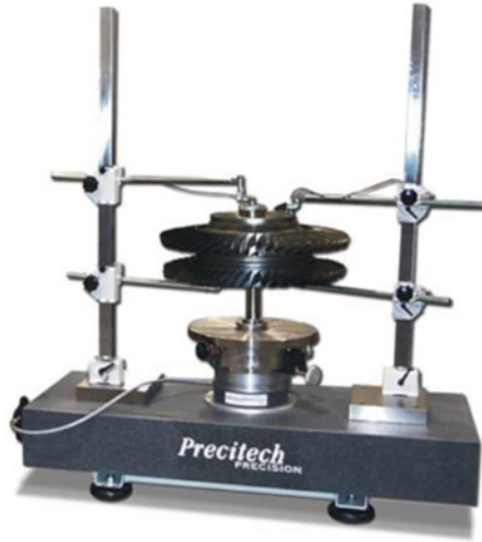
Fig. 1. The part measurement and stacking prediction system.
