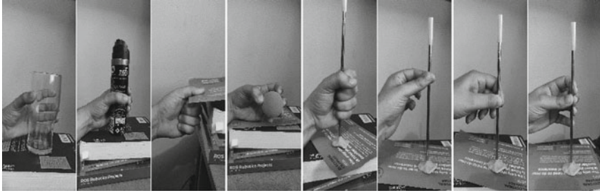
Fig. 4 Functional grasps performed: top row (from left to right). 1. Power grasp, 2. Medium wrap, 3. Lateral grasp, 4. Precision sphere, 5. Small diameter grasp, 6. Tip pinch, 7. Writing tripod, 8. Prismatic quad grasp
