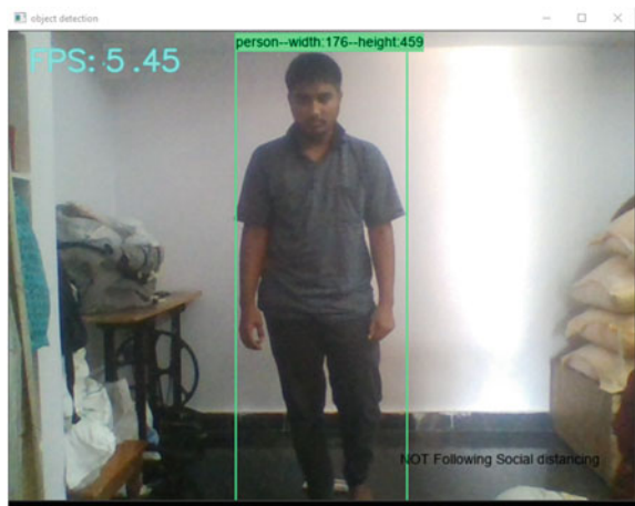
Fig. 11 Detection of person and showing alert on the screen as person is not at the distance of six feet from the user
