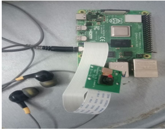
Fig. 2 Proposed prototype. Raspberry Pi with the camera module and headphones
