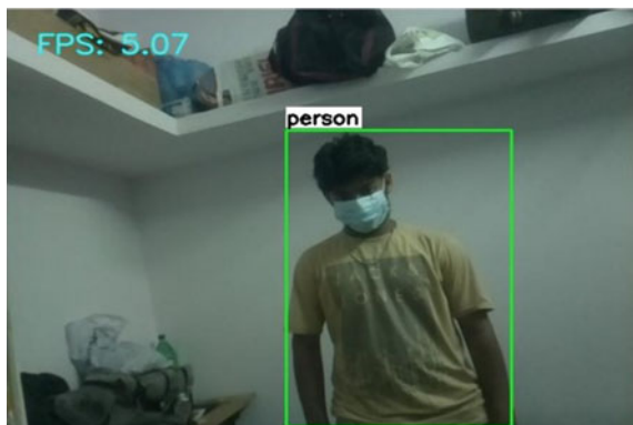
Fig. 9 Detection of person using optimized model deployed in Raspberry Pi
