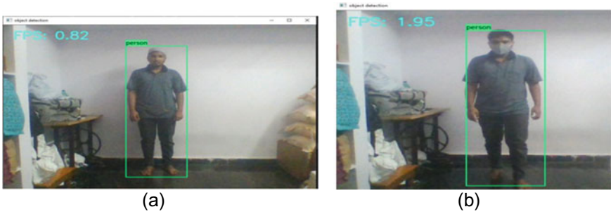
Fig. 8 a Detection model implemented with SSD VGG16 Net b detection model implemented with SSD MobileNet
