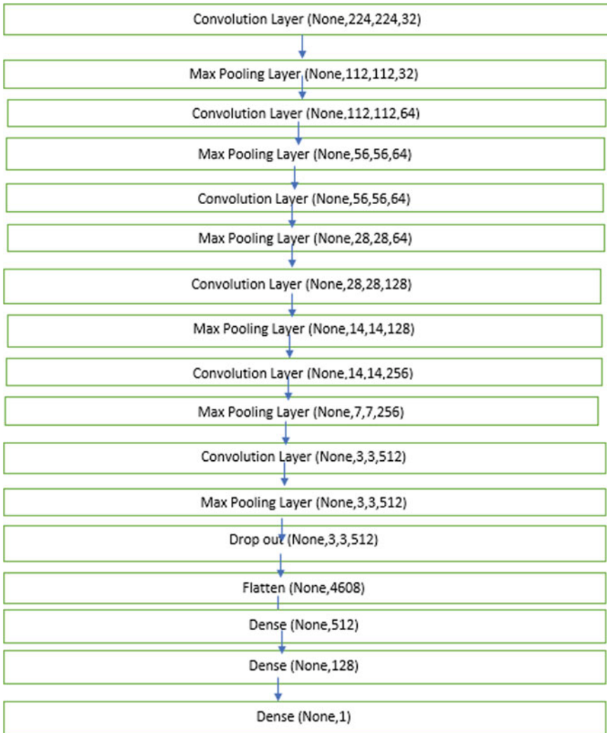
Fig. 7 CNN architecture model for hard exudates detection
