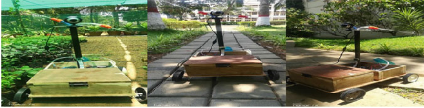
Fig. 10 a Autonomous robot sprinkling water with crop detection using SVM linear image classifier. b Autonomous robot sprinkling water with lane detection. c Autonomous robot sprinkling water
