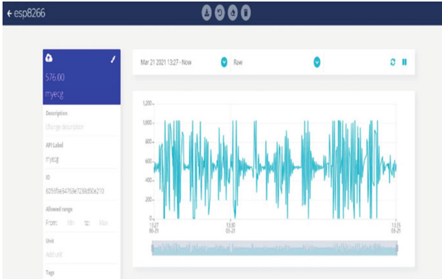
Fig. 4 (As observed in Fig. 4), the ECG graph with P, Q, R, S, T points is plotted directly on cloud. This allows the doctor to observe the graph and make accurate deductions regarding the patients’ health. You can also observe the dashboard, which can help the patient and doctor to design and adjust it in a way convenient to them
