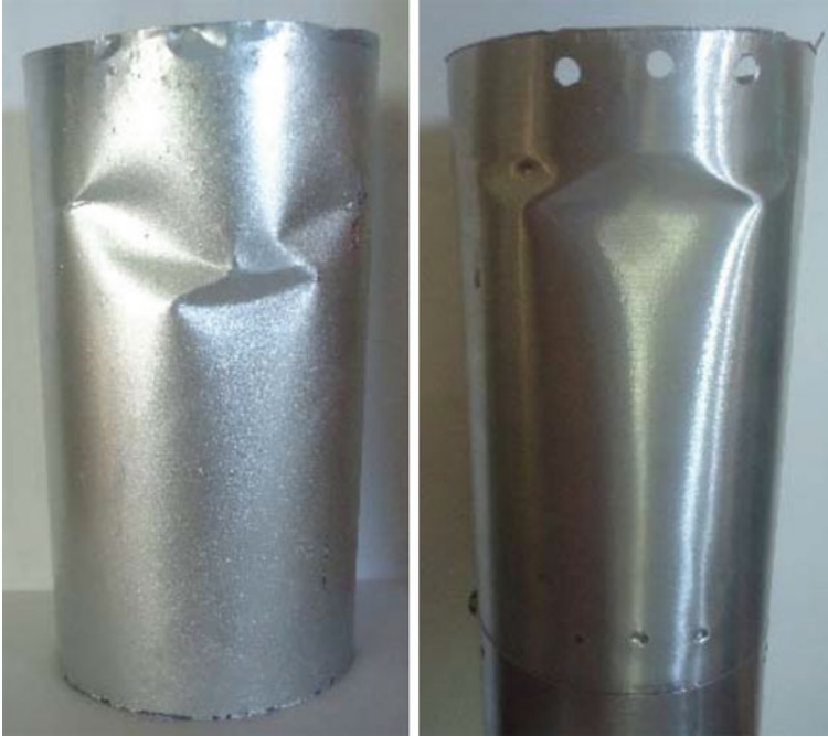
Fig. 3 Shape of shells after loss of stability
